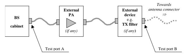
Figure 4.10.1-1: Transmitter test ports
