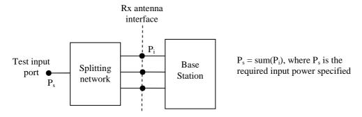
Figure 4.10.7.1-1: Receiver test set-up
