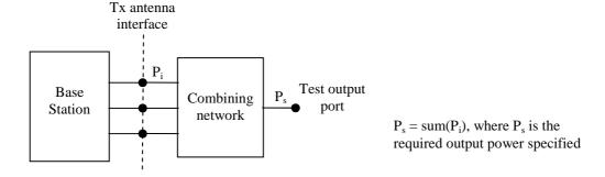
Figure 4.10.7.2-1: Transmitter test set-up
