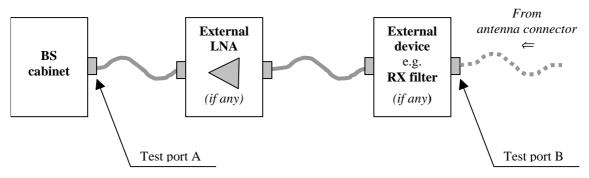
Figure 4.10.2-1: Receiver test ports
