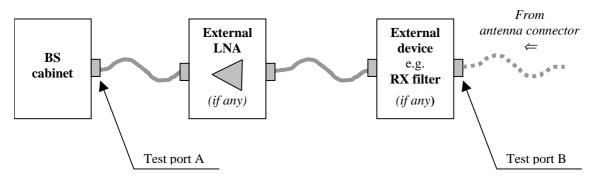
Figure 7.1-1: Receiver test ports
