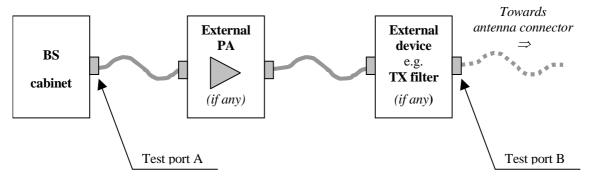
Figure 6.1-1: Transmitter test ports
