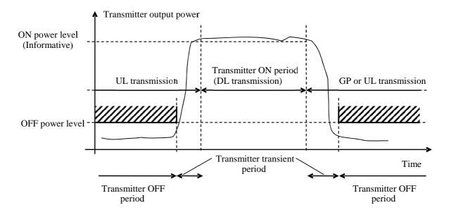
Figure 6.4.2-2: Illustration of the relations of transmitter ON period, transmitter OFF period and transmitter transient period (for NR)
