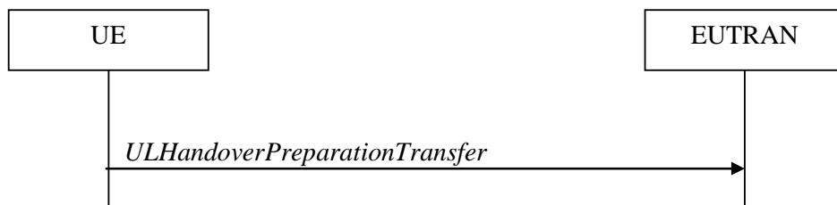
Figure 5.4.5.1-1: UL handover preparation transfer
