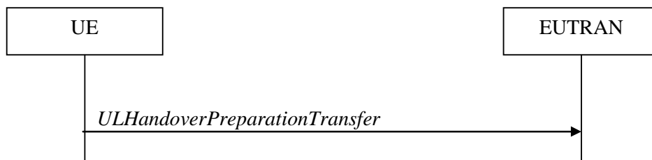
Figure 5.4.5.1-1: UL handover preparation transfer
