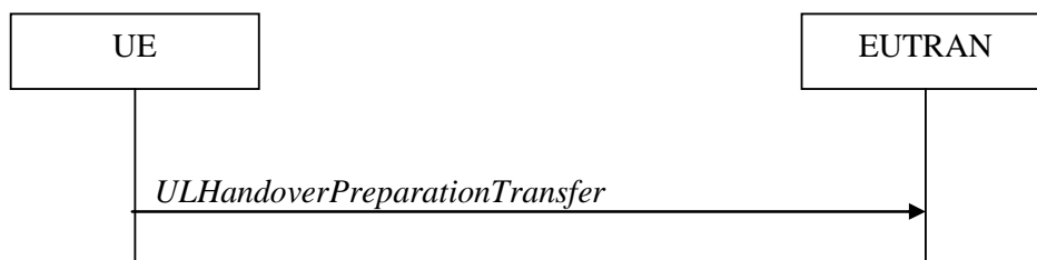
Figure 5.4.5.1-1: UL handover preparation transfer
