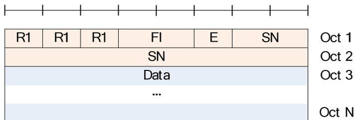
Figure 6.2.1.3-2: UMD PDU with 10 bit SN (No LI)
