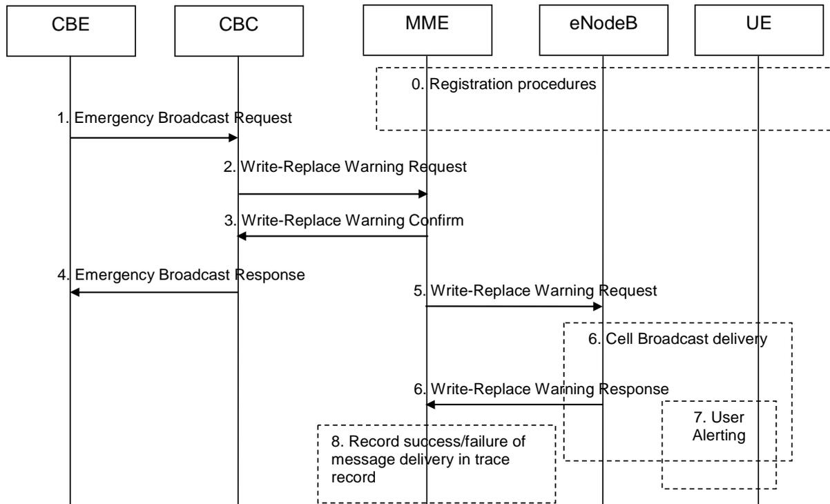
**Figure 9.1.3.4.2-1: Warning message delivery procedure in E-UTRAN**
