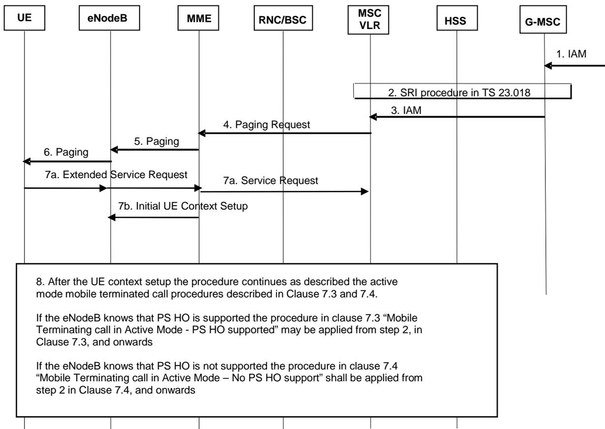
Figure 7.2-1: Mobile Terminating Call in idle mode
