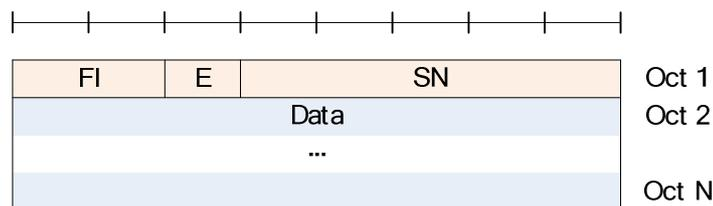
**Figure 6.2.1.3-1: UMD PDU with 5 bit SN (No LI)**
