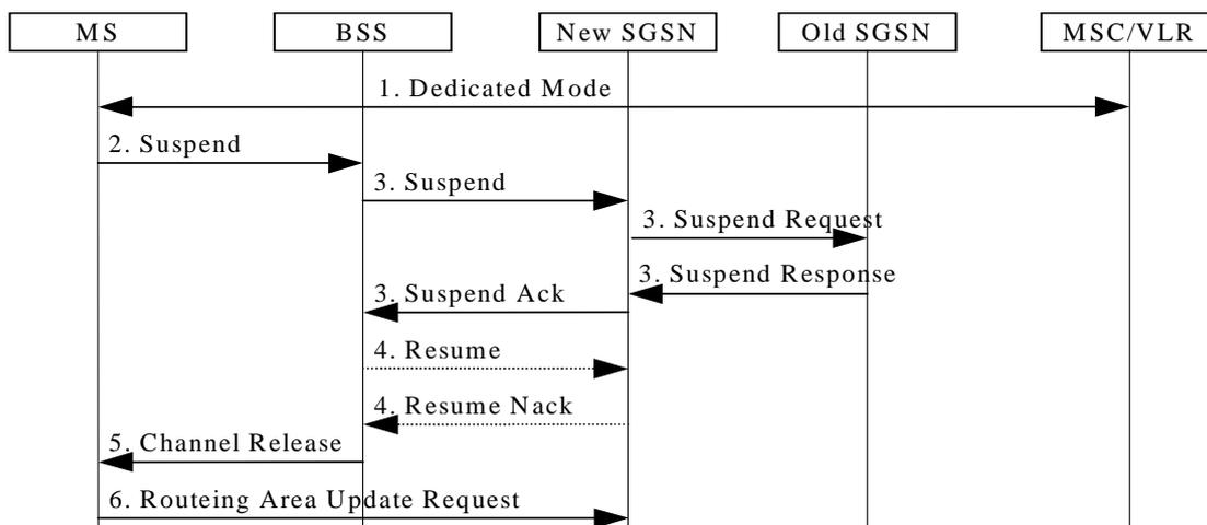
**Figure 100: Suspend and Resume Procedure for inter-SGSN**
