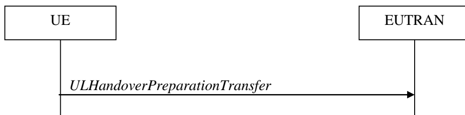
Figure 5.4.5.1-1: UL handover preparation transfer
