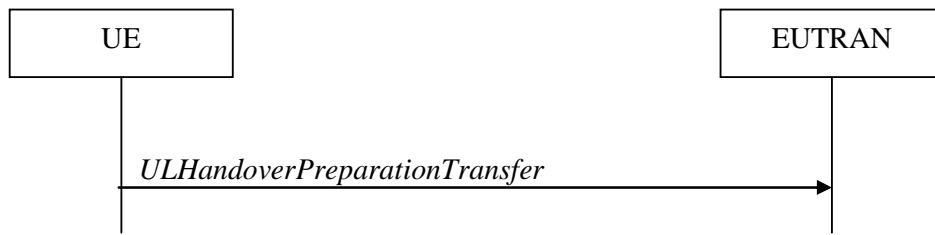
Figure 5.4.5.1-1: UL handover preparation transfer
