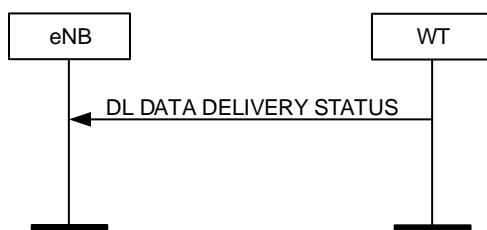
Figure 5.4.2.1-1: Successful Downlink Data Delivery Status
