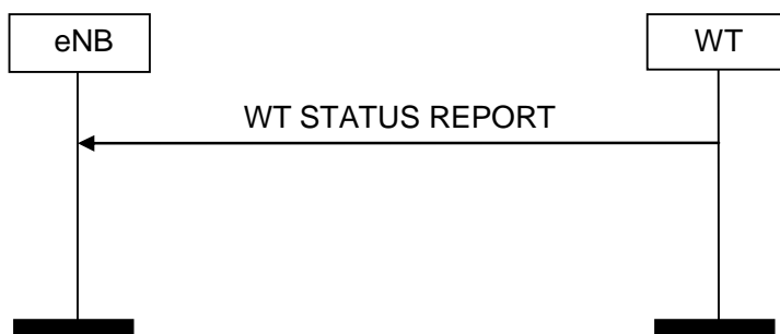
Figure 8.5.2-1: WT Status Reporting procedure, successful operation
