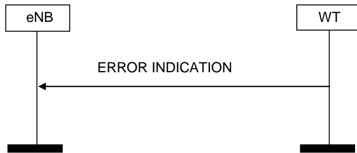
Figure 8.6.2-2: Error Indication procedure, WT originated. Successful operation.
