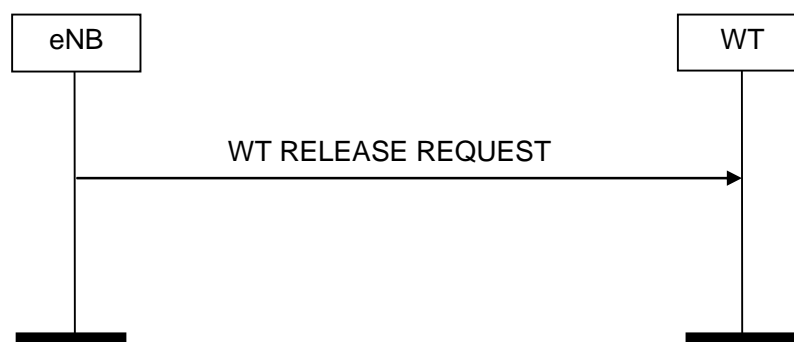
Figure 8.11.2-1: eNB initiated WT Release, successful operation
