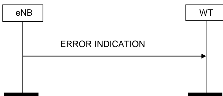
Figure 8.6.2-1: Error Indication procedure, eNB originated. Successful operation.
