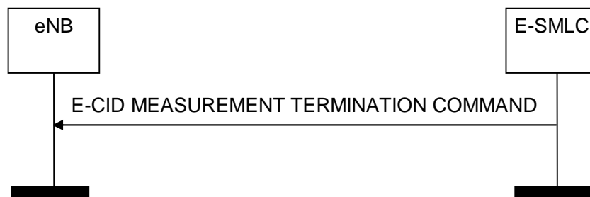
Figure 8.2.4.2-1: E-CID Measurement Termination procedure, successful operation
