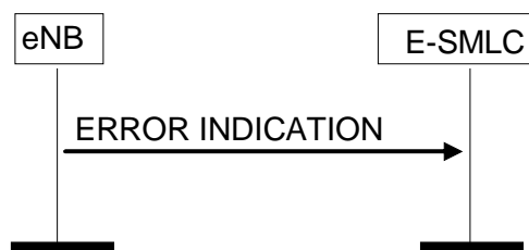
Figure 8.3.1.2-2: Error Indication procedure, eNB originated, successful operation
