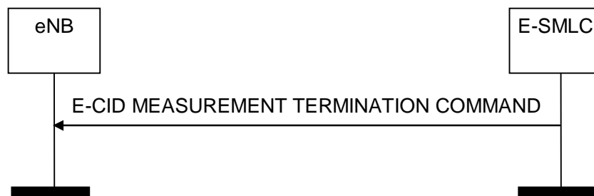
Figure 8.2.4.2-1: E-CID Measurement Termination procedure, successful operation
