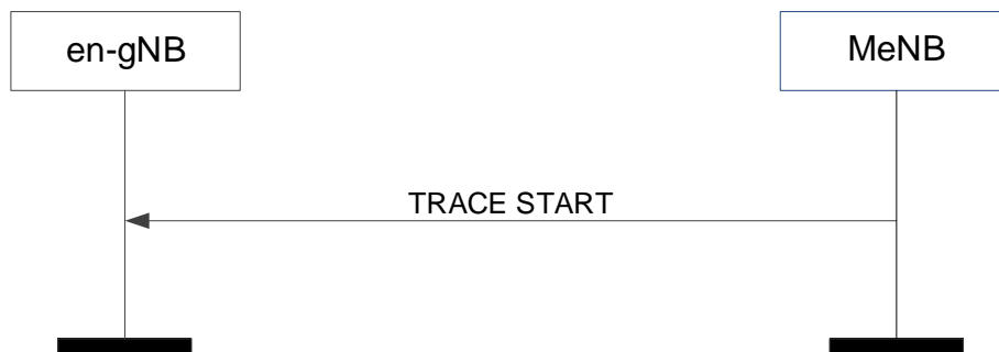
Figure 8.7.19.2-1: Trace Start, successful operation
