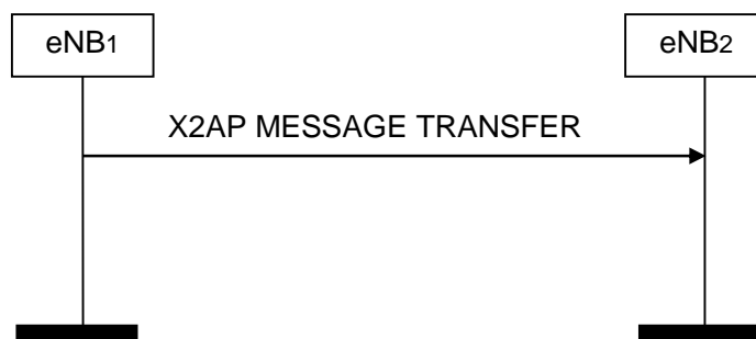
Figure 8.5.2-1: X2AP Message Transfer, successful operation
