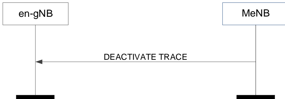
Figure 8.7.20.2-1: Deactivate Trace, successful operation
