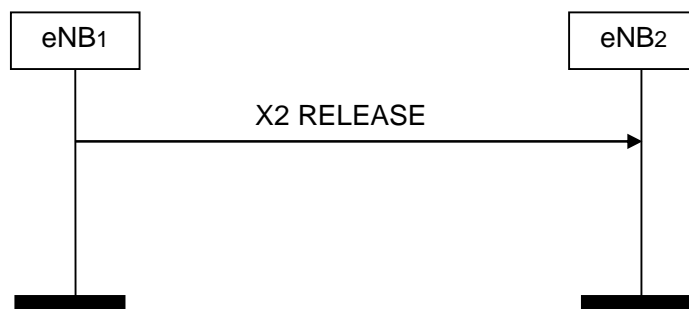
Figure 8.4.2-1: X2AP Release, successful operation
