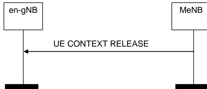
Figure 8.2.3.2-3: UE Context Release, successful operation for EN-DC
