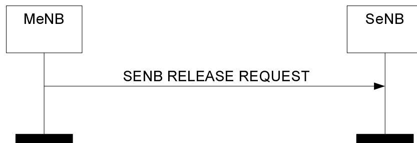
Figure 8.6.5.2-1: MeNB initiated SeNB Release, successful operation
