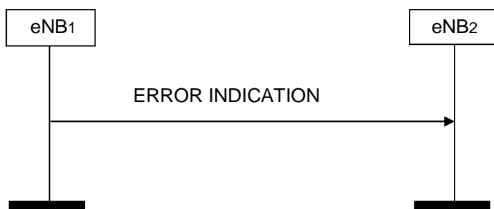
Figure 8.3.2.2-1: Error Indication, successful operation.
