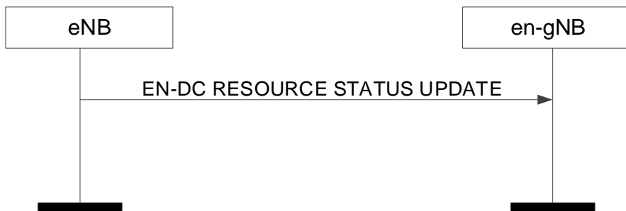
Figure 8.7.22.2-2: EN-DC Resource Status Reporting, successful operation - eNB-initiated
