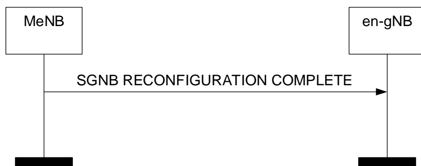
Figure 8.7.5.2-1: SgNB Reconfiguration Complete procedure, successful operation.
