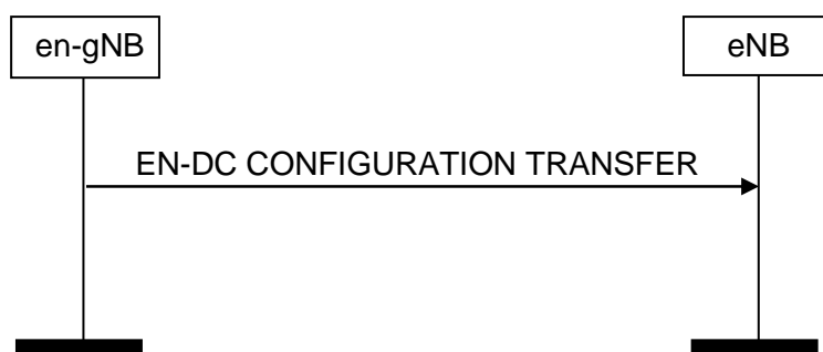
Figure 8.7.18.2-2: en-gNB initiated EN-DC Configuration Transfer, successful operation
