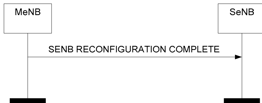
Figure 8.6.2.2-1: SeNB Reconfiguration Complete procedure, successful operation.
