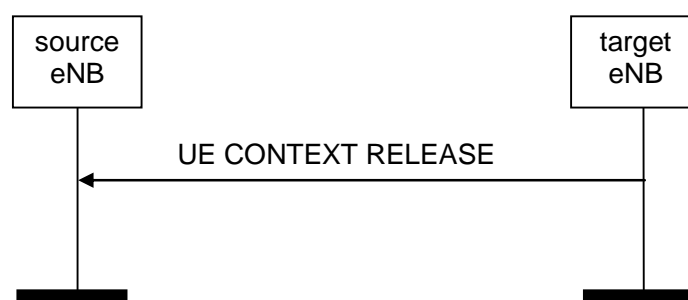
Figure 8.2.3.2-1: UE Context Release, successful operation for handover
