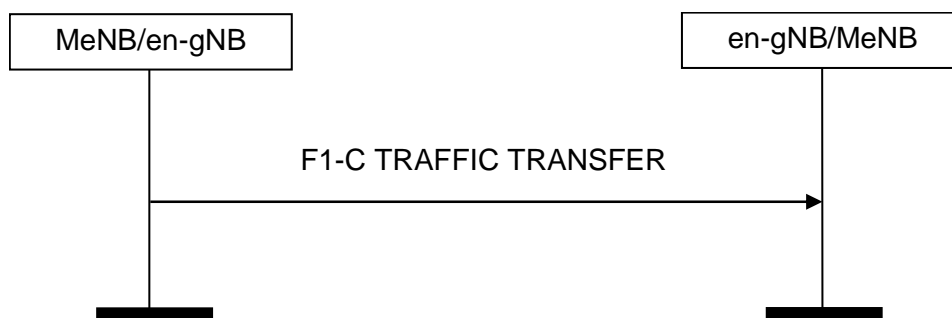
Figure 8.8.1.2-1: F1-C Traffic Transfer procedure, successful operation.
