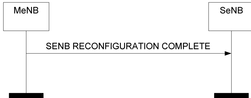
Figure 8.6.2.2-1: SeNB Reconfiguration Complete procedure, successful operation.
