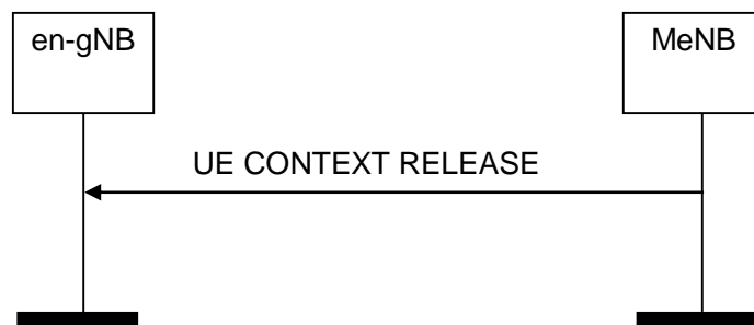
Figure 8.2.3.2-3: UE Context Release, successful operation for EN-DC
