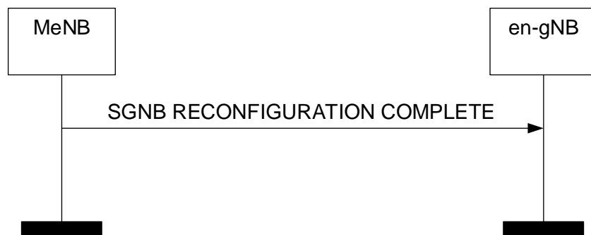
Figure 8.7.5.2-1: SgNB Reconfiguration Complete procedure, successful operation.
