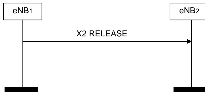
Figure 8.4.2-1: X2AP Release, successful operation
