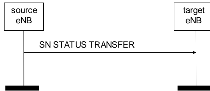
Figure 8.2.2.2-1: SN Status Transfer, successful operation
