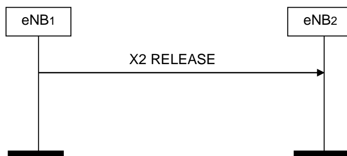
Figure 8.4.2-1: X2AP Release, successful operation
