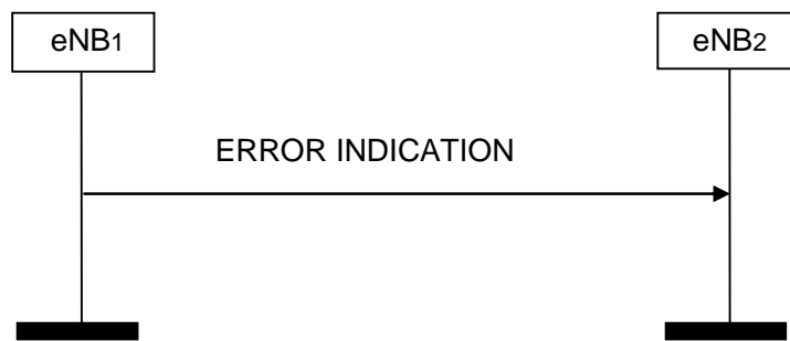
Figure 8.3.2.2-1: Error Indication, successful operation.
