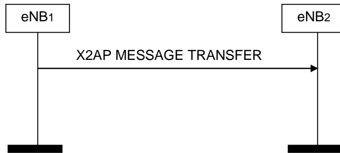
Figure 8.5.2-1: X2AP Message Transfer, successful operation
