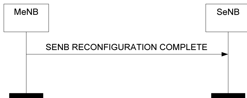
Figure 8.6.2.2-1: SeNB Reconfiguration Complete procedure, successful operation.
