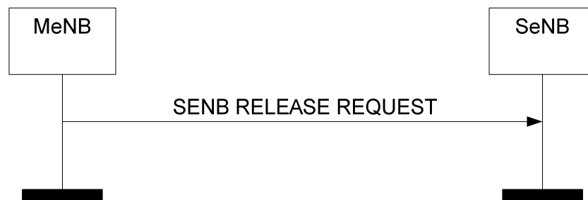
Figure 8.6.5.2-1: MeNB initiated SeNB Release, successful operation
