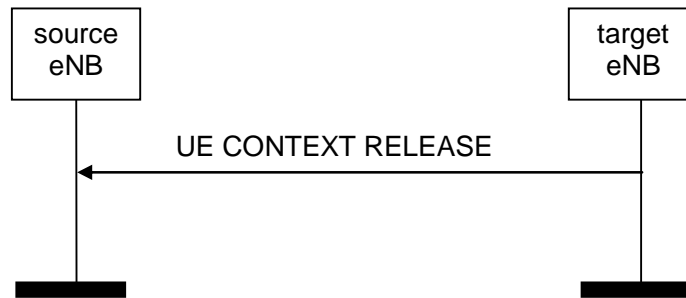
Figure 8.2.3.2-1: UE Context Release, successful operation for handover
