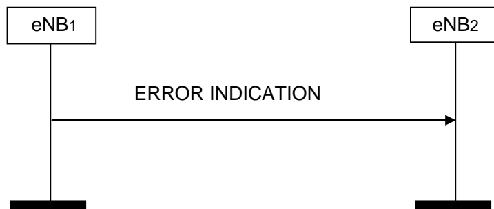
Figure 8.3.2.2-1: Error Indication, successful operation.
