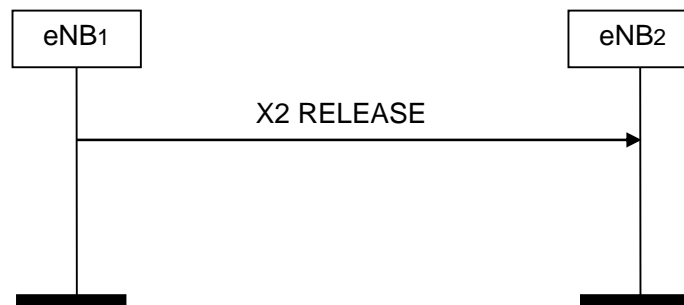
Figure 8.4.2-1: X2AP Release, successful operation
