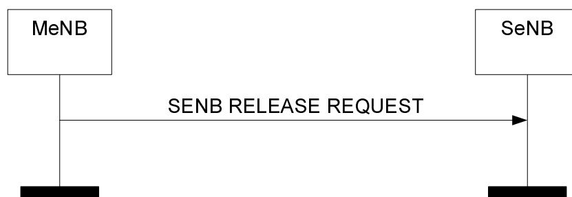
Figure 8.6.5.2-1: MeNB initiated SeNB Release, successful operation
