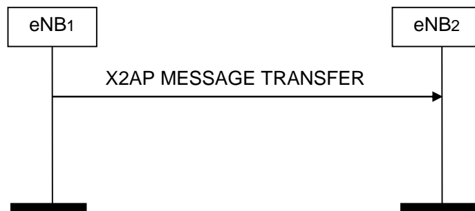
Figure 8.5.2-1: X2AP Message Transfer, successful operation
