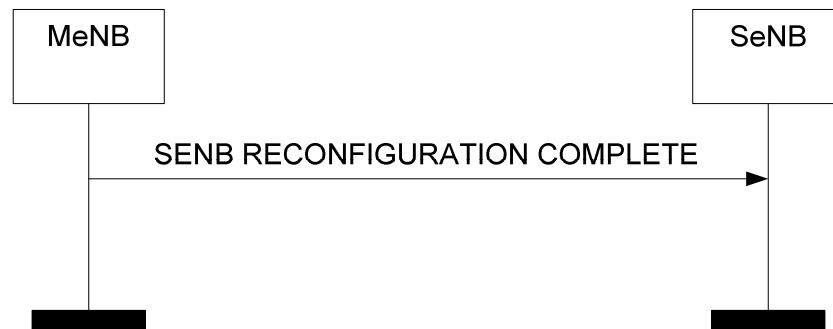
Figure 8.6.2.2-1: SeNB Reconfiguration Complete procedure, successful operation.
