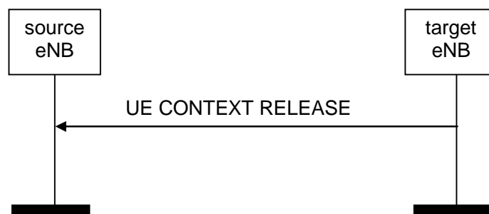
Figure 8.2.3.2-1: UE Context Release, successful operation for handover
