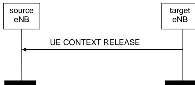
Figure 8.2.3.2-1: UE Context Release, successful operation
