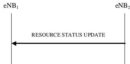
Figure 8.3.7.2-1: Resource Status Reporting, successful operation
