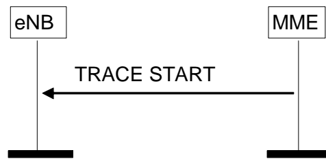
Figure 8.10.1.2-1: Trace Start procedure.
