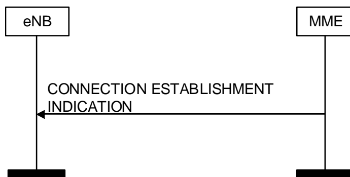
Figure 8.3.9.2-1: Connection Establishment Indication procedure. Successful operation.
