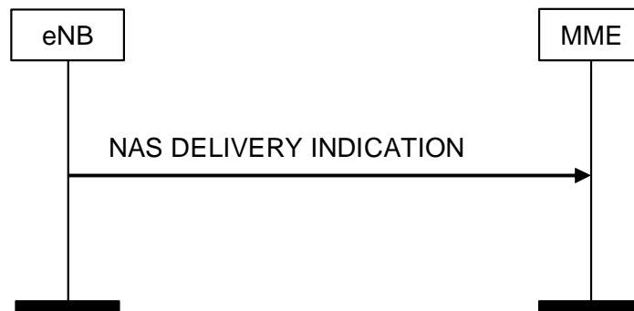
Figure 8.6.2.4a-1: NAS DELIVERY INDICATION Procedure
