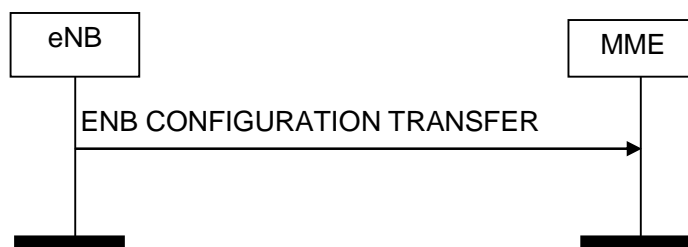
Figure 8.15.2.1-1: eNB Configuration Transfer procedure. Successful operation.
