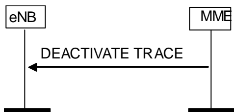
Figure 8.10.3.2-1: Deactivate Trace procedure. Successful operation.
