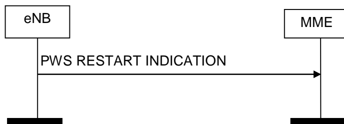
Figure 8.12.3.2-1: PWS Restart Indication procedure. Successful operation.
