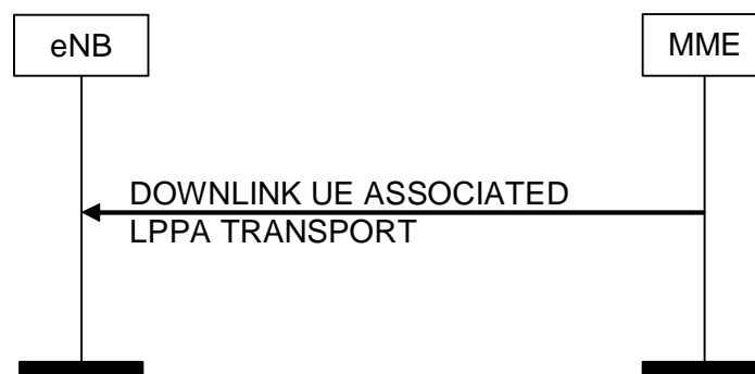
Figure 8.17.2.1-1: DOWNLINK UE ASSOCIATED LPPA Transport Procedure
