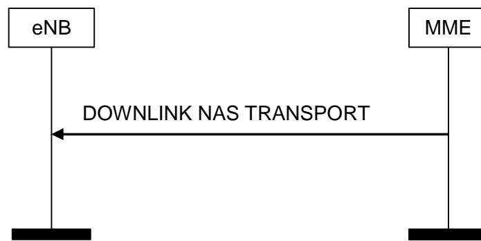
Figure 8.6.2.2-1: DOWNLINK NAS Transport Procedure
