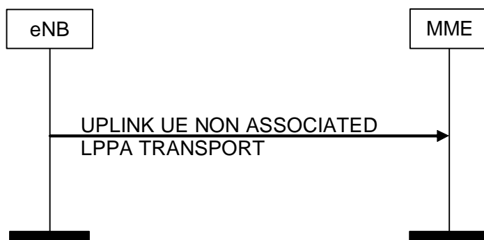
Figure 8.17.2.4-1: UPLINK NON UE ASSOCIATED LPPA TRANSPORT Procedure
