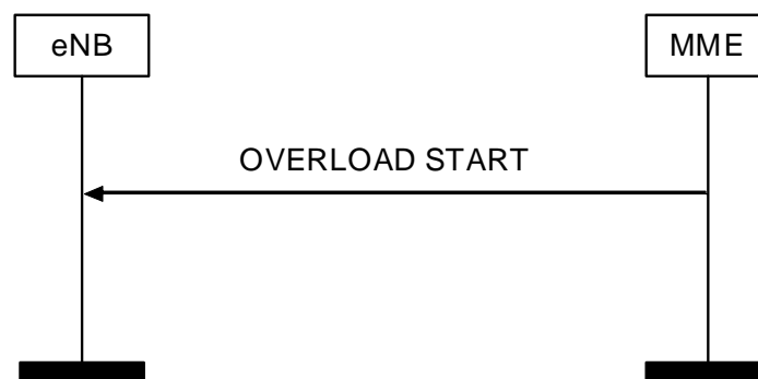
Figure 8.7.6.2-1: Overload Start procedure
