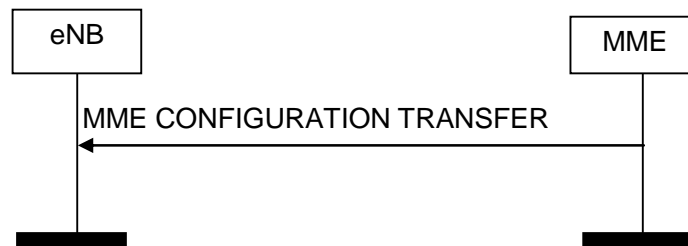
Figure 8.16.2.1-1: MME Configuration Transfer procedure. Successful operation.
