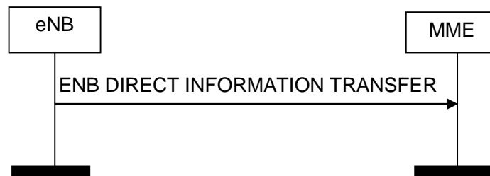
Figure 8.13.1.2-1: ENB Direct Information Transfer procedure. Successful operation.
