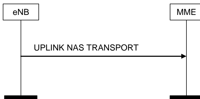
Figure 8.6.2.3-1: UPLINK NAS TRANSPORT Procedure
