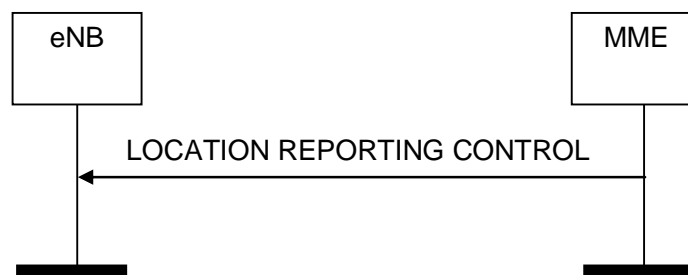
Figure 8.11.1.2-1: Location Reporting Control procedure. Successful operation.
