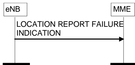
Figure 8.11.2.2-1: Location Report Failure Indication procedure.
