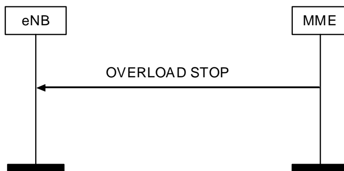
Figure 8.7.7.2.-1: Overload Stop procedure
