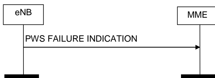
Figure 8.12.4.2-1: PWS Failure Indication procedure. Successful operation.
