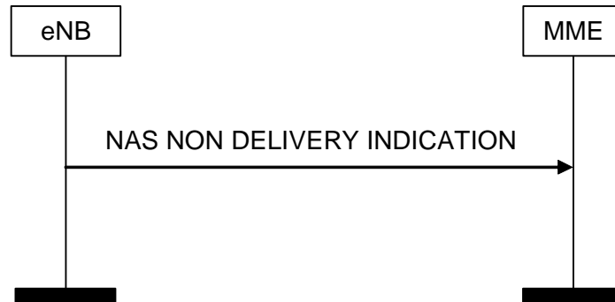
Figure 8.6.2.4-1: NAS NON DELIVERY INDICATION Procedure
