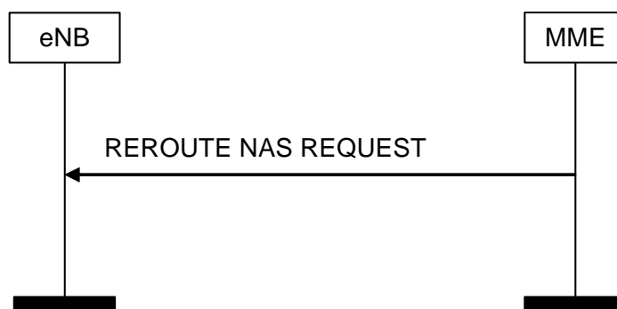
Figure 8.6.2.5-1: Reroute NAS Request Procedure
