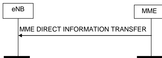
Figure 8.14.1.2-1: MME Direct Information Transfer procedure. Successful operation.
