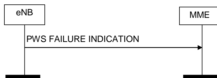
Figure 8.12.4.2-1: PWS Failure Indication procedure. Successful operation.
