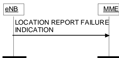
Figure 8.11.2.2-1: Location Report Failure Indication procedure.
