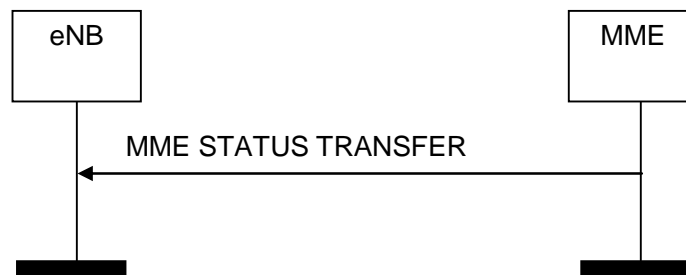
Figure 8.4.7.2-1: MME Status Transfer procedure
