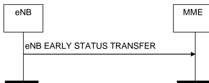
Figure 8.4.9.2-1: eNB Early Status Transfer procedure
