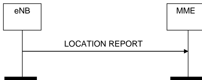
Figure 8.11.3.2-1: Location Report procedure. Successful operation.
