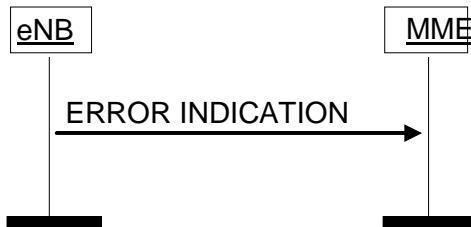
**Figure 8.7.2.2-2: Error Indication procedure, eNB originated. Successful operation.**
