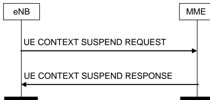
**Figure 8.3.7.2-1: UE Context Suspend procedure. Successful operation.**
