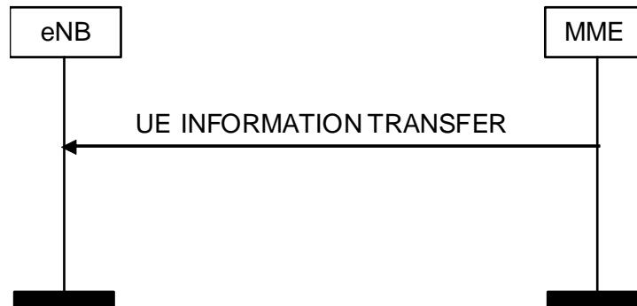
**Figure 8.3.11.1: UE Information Transfer Procedure. Successful operation.**
