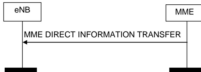
**Figure 8.14.1.2-1: MME Direct Information Transfer procedure. Successful operation.**
