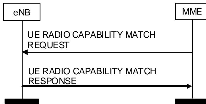
**Figure 8.3.5.2-1: UE Radio Capability Match. Successful operation**
