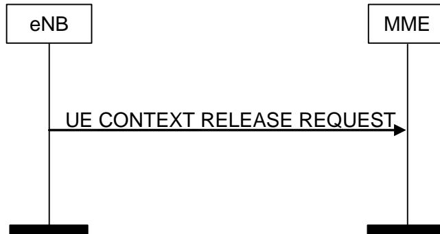
**Figure 8.3.2.2-1: UE Context Release Request procedure. Successful operation.**
