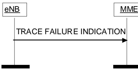
**Figure 8.10.2.2-1: Trace Failure Indication procedure.**
