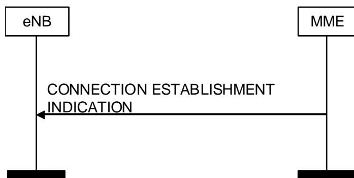
**Figure 8.3.9.2-1: Connection Establishment Indication procedure. Successful operation.**
