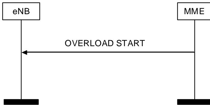
**Figure 8.7.6.2-1: Overload Start procedure**
