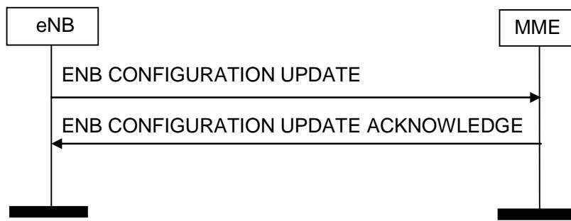
**Figure 8.7.4.2-1: ENB Configuration Update procedure: Successful Operation.**
