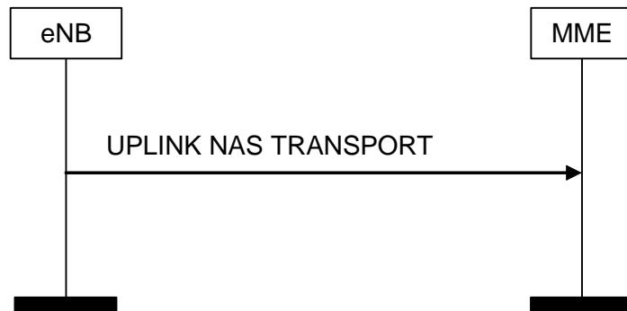
**Figure 8.6.2.3-1: UPLINK NAS TRANSPORT Procedure**
