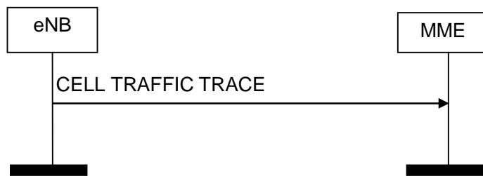
**Figure 8.10.4.2-1: Cell Traffic Trace procedure. Successful operation.**
