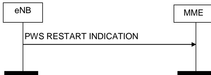
**Figure 8.12.3.2-1: PWS Restart Indication procedure. Successful operation.**
