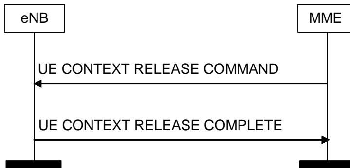
**Figure 8.3.3.2-1: UE Context Release procedure. Successful operation.**
