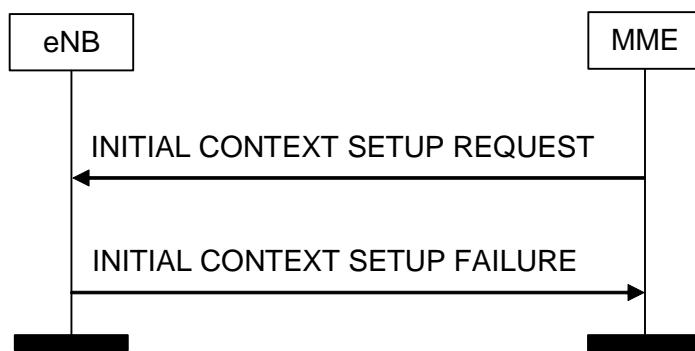
**Figure 8.3.1.3-1: Initial Context Setup procedure. Unsuccessful operation.**
