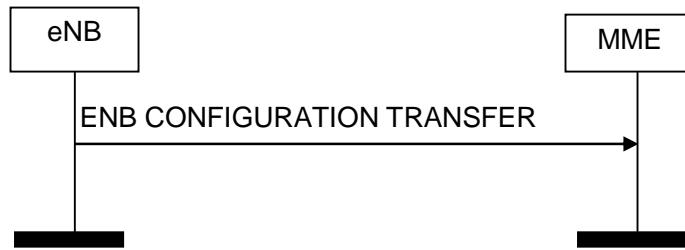
**Figure 8.15.2.1-1: eNB Configuration Transfer procedure. Successful operation.**
