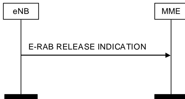
**Figure 8.2.3.2.2-1: E-RAB Release INDICATION procedure. Successful operation.**
