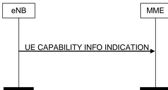
**Figure 8.9.2-1: UE Capability Info Indication procedure. Successful operation.**
