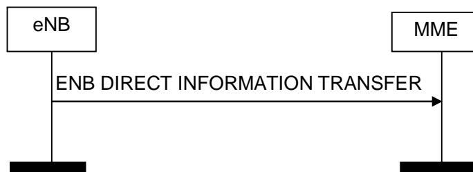
**Figure 8.13.1.2-1: ENB Direct Information Transfer procedure. Successful operation.**
