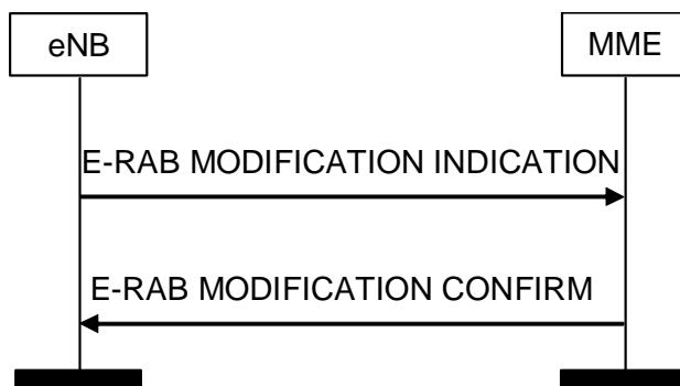
**Figure 8.2.4.2-1: E-RAB Modification Indication procedure. Successful operation.**
