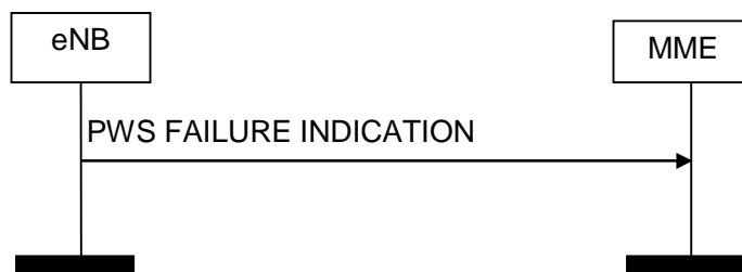
**Figure 8.12.4.2-1: PWS Failure Indication procedure. Successful operation.**
