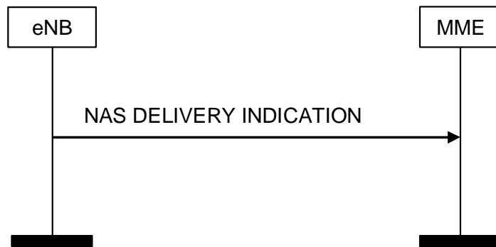
**Figure 8.6.2.4a-1: NAS DELIVERY INDICATION Procedure**
