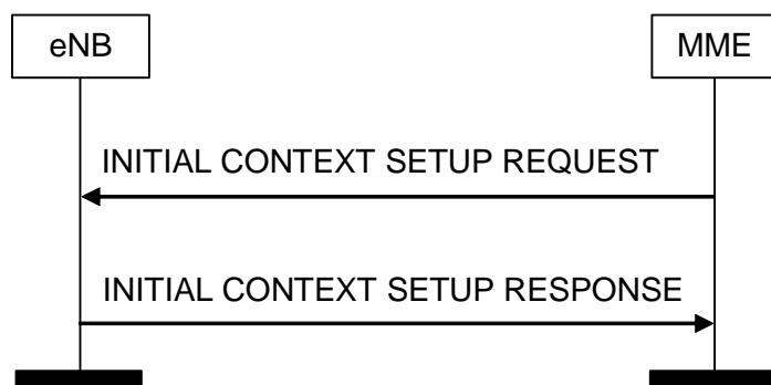
**Figure 8.3.1.2-1: Initial Context Setup procedure. Successful operation.**
