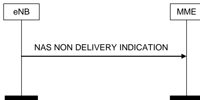
Figure 8.6.2.4-1: NAS NON DELIVERY INDICATION Procedure
