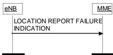
Figure 8.11.2.2-1: Location Report Failure Indication procedure.
