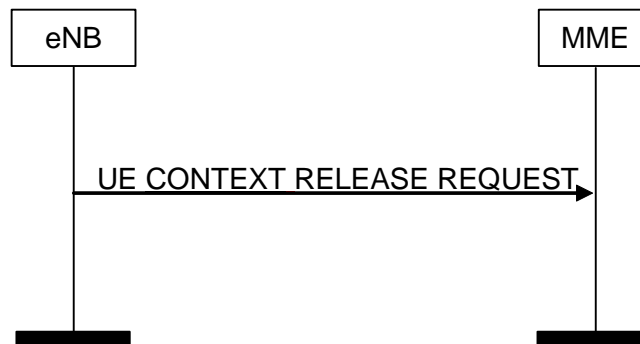
Figure 8.3.2.2-1: UE Context Release Request procedure. Successful operation.
