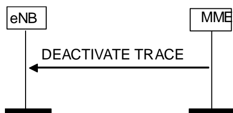
Figure 8.10.3.2-1: Deactivate Trace procedure. Successful operation.
