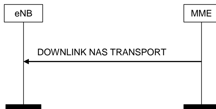
Figure 8.6.2.2-1: DOWNLINK NAS Transport Procedure
