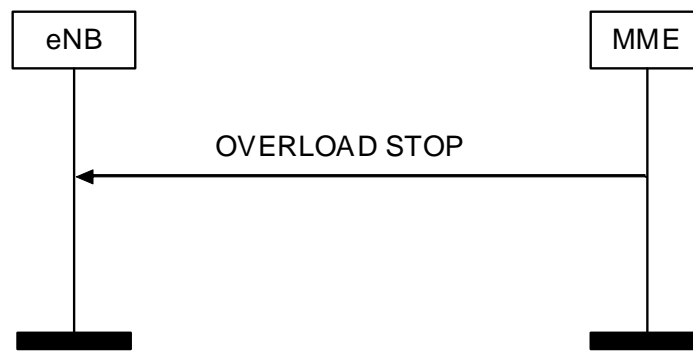
Figure 8.7.7.2.-1: Overload Stop procedure
