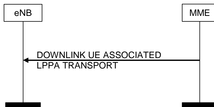
Figure 8.17.2.1-1: DOWNLINK UE ASSOCIATED LPPA Transport Procedure
