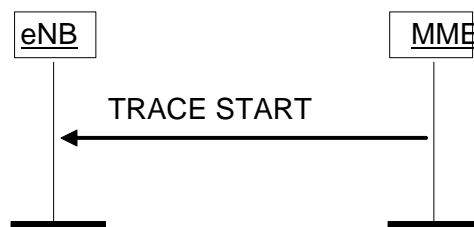
Figure 8.10.1.2-1: Trace Start procedure.
