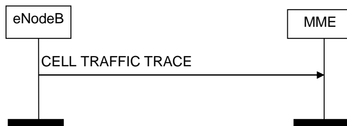
Figure 8.10.4.2-1: Cell Traffic Trace procedure. Successful operation.
