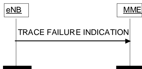
Figure 8.10.2.2-1: Trace Failure Indication procedure.
