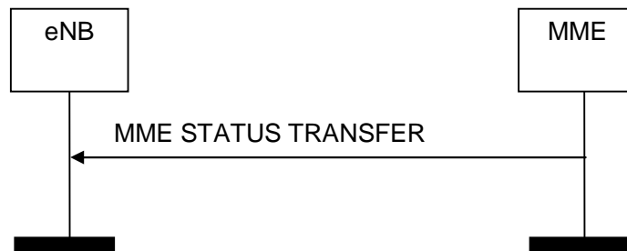
Figure 8.4.7.2-1: MME Status Transfer procedure
