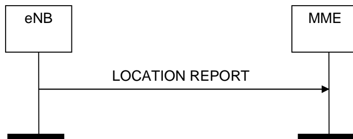
Figure 8.11.3.2-1: Location Report procedure. Successful operation.
