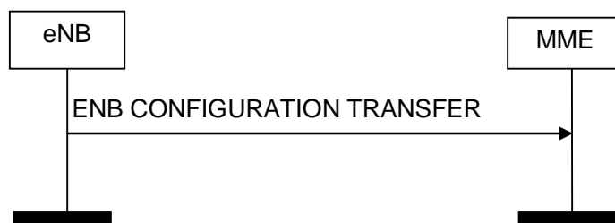
Figure 8.15.2.1-1: eNB Configuration Transfer procedure. Successful operation.
