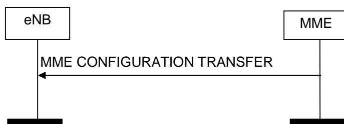
Figure 8.16.2.1-1: MME Configuration Transfer procedure. Successful operation.
