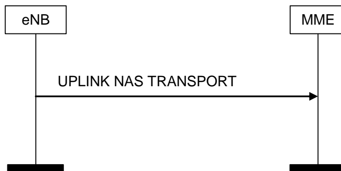
Figure 8.6.2.3-1: UPLINK NAS TRANSPORT Procedure
