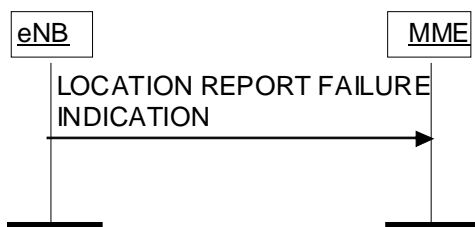
Figure 8.11.2.2-1: Location Report Failure Indication procedure.
