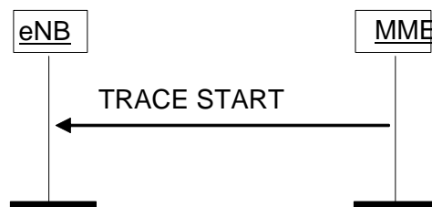
Figure 8.10.1.2-1: Trace Start procedure.
