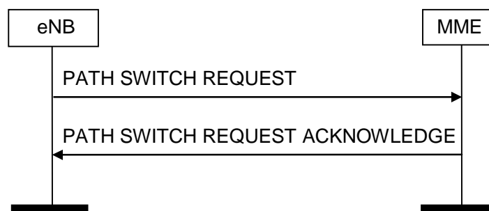
Figure 8.4.4.2-1: Path switch request: successful operation
