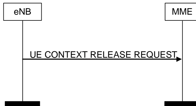
Figure 8.3.2.2-1: UE Context Release Request procedure. Successful operation.
