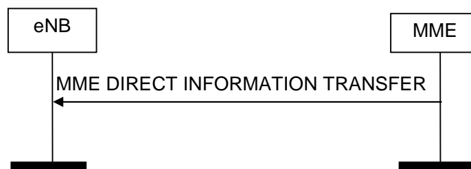
Figure 8.14.1.2-1: MME Direct Information Transfer procedure. Successful operation.
