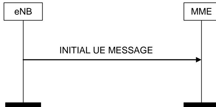
Figure 8.6.2.1-1: Initial UE Message procedure
