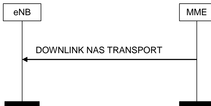
Figure 8.6.2.2-1: DOWNLINK NAS Transport Procedure
