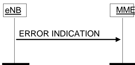
Figure 8.7.2.2-2: Error Indication procedure, eNB originated. Successful operation.
