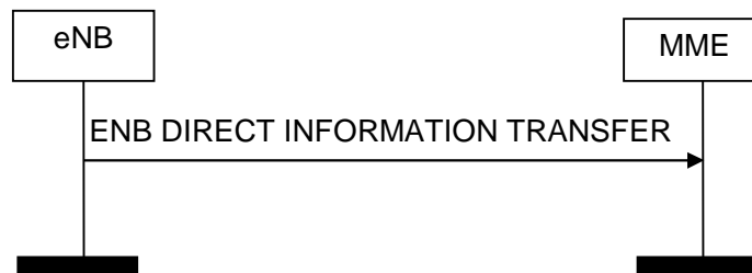
Figure 8.13.1.2-1: ENB Direct Information Transfer procedure. Successful operation.
