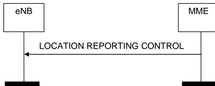
Figure 8.11.1.2-1: Location Reporting Control procedure. Successful operation.
