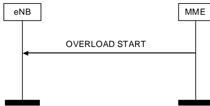
Figure 8.7.6.2-1: Overload Start procedure
