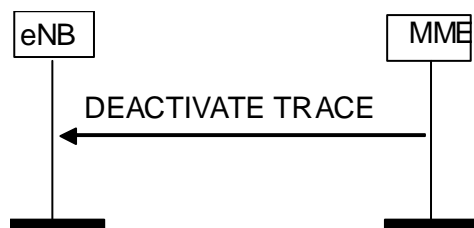
Figure 8.10.3.2-1: Deactivate Trace procedure. Successful operation.
