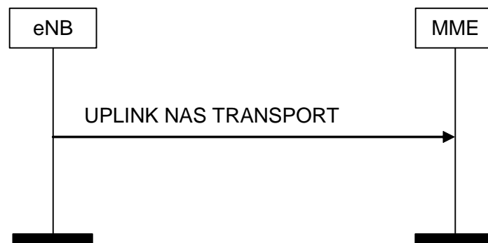
Figure 8.6.2.3-1: UPLINK NAS TRANSPORT Procedure
