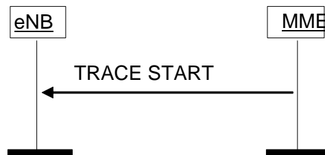
Figure 8.10.1.2-1: Trace Start procedure.
