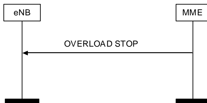
Figure 8.7.7.2-1: Overload Stop procedure
