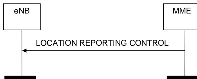
Figure 8.11.1.2-1: Location Reporting Control procedure. Successful operation.
