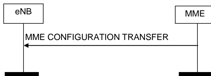
Figure 8.16.2.1-1: MME Configuration Transfer procedure. Successful operation.
