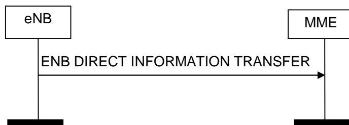
Figure 8.13.1.2-1: ENB Direct Information Transfer procedure. Successful operation.
