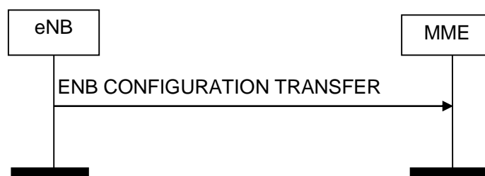
Figure 8.15.2.1-1: eNB Configuration Transfer procedure. Successful operation.
