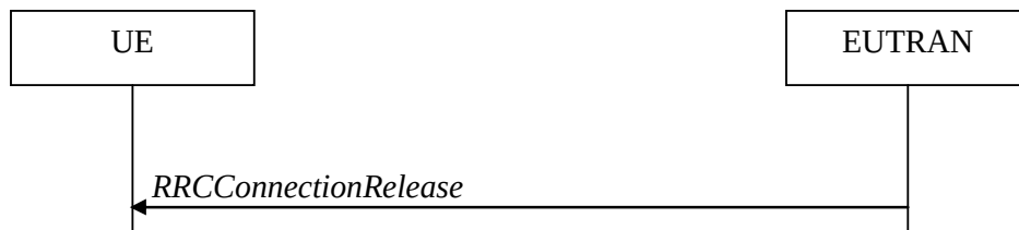
Figure 5.3.8.1-1: RRC connection release, successful
