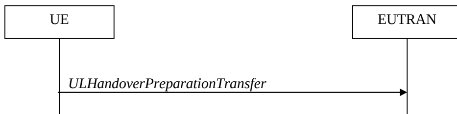
Figure 5.4.5.1-1: UL handover preparation transfer
