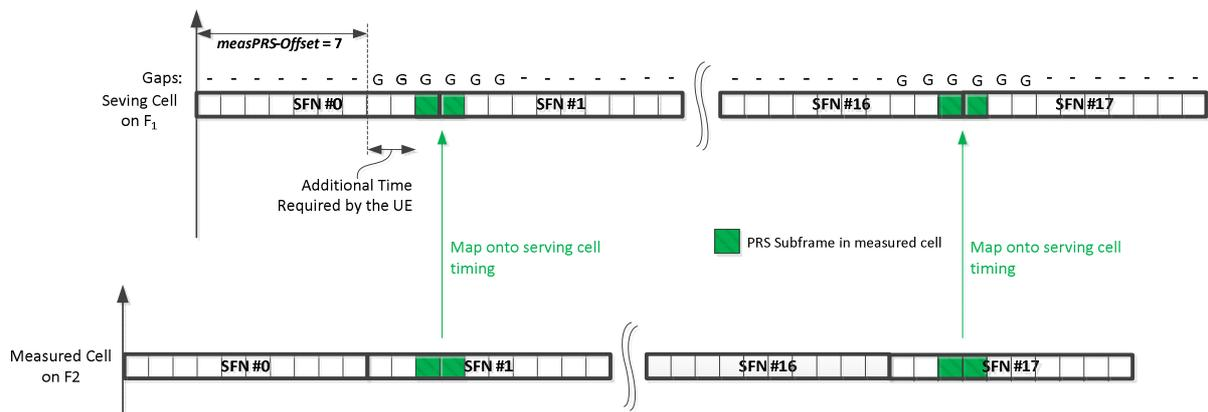
Figure 6.2.2-1 (informative): Exemplary calculation of *measPRS-Offset* field.
