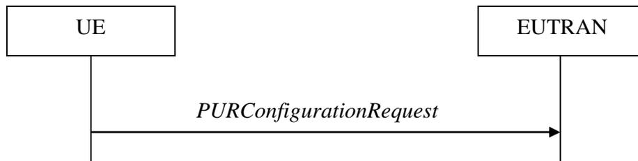
**Figure 5.6.23.1-1: PUR Configuration Request**
