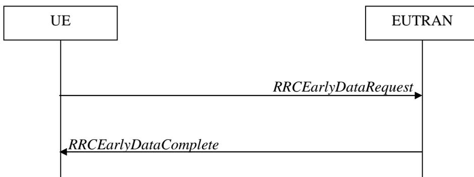
Figure 5.3.3.1-7: CP-EDT or CP transmission using PUR, successful
