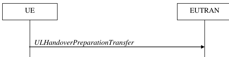
Figure 5.4.5.1-1: UL handover preparation transfer
