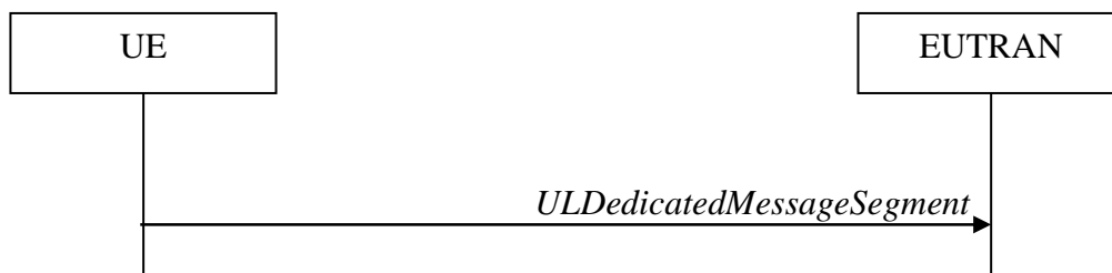
Figure 5.6.22.1-1: UL message segment transfer
