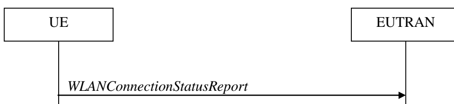
Figure 5.6.15.2.1-1: WLAN connection status reporting
