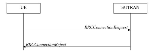
Figure 5.3.3.1-2: RRC connection establishment, network reject
