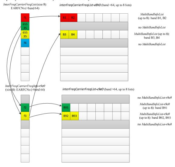
Figure D.1.2-1: Mapping of EARFCNs to MultiBandInfoList/MultiBandInfoList-v9e0
