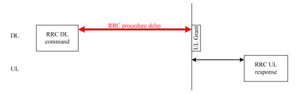
Figure 11.2-1: Illustration of RRC procedure delay
