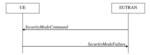
Figure 5.3.4.1-2: Security mode command, failure
