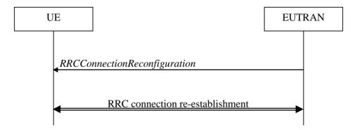
Figure 5.3.5.1-2: RRC connection reconfiguration, failure
