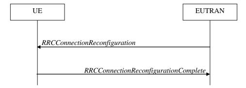
Figure 5.3.5.1-1: RRC connection reconfiguration, successful
