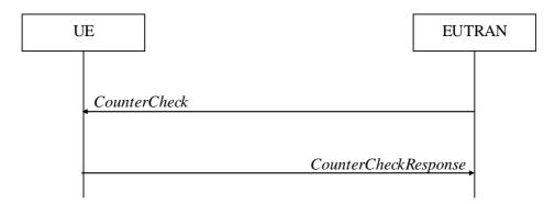
Figure 5.3.6.1-1: Counter check procedure
