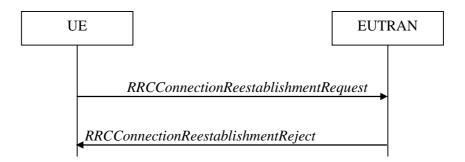
Figure 5.3.7.1-2: RRC connection re-establishment, failure
