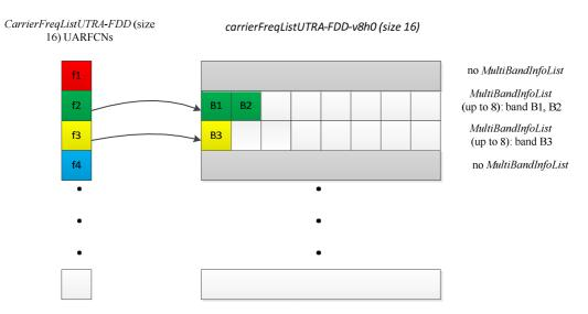
Figure D.1.3-1: Mapping of UARFCNs to MultiBandInfoList
