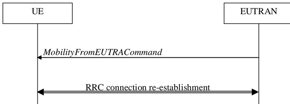
Figure 5.4.3.1-2: Mobility from E-UTRA, failure
