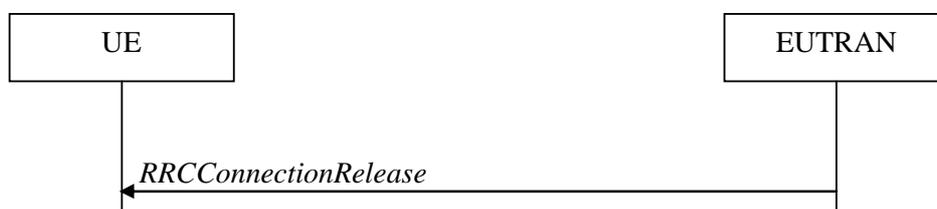
**Figure 5.3.8.1-1: RRC connection release, successful**
