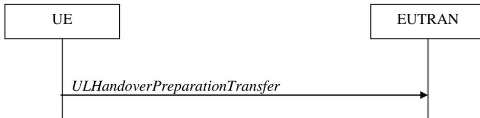
**Figure 5.4.5.1-1: UL handover preparation transfer**
