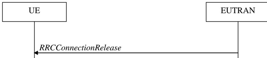
**Figure 5.3.8.1-1: RRC connection release, successful**
