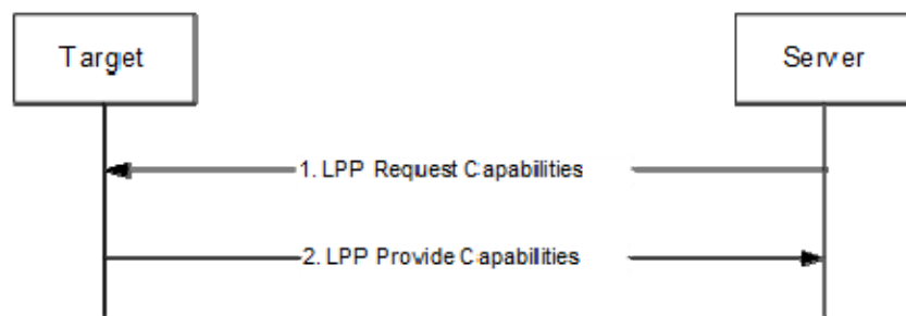
Figure 7.1.2.1-1: LPP Capability Transfer procedure
