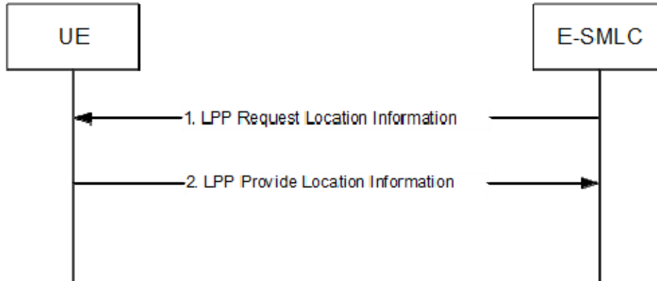
Figure 8.2.3.3.1-1: E-SMLC-initiated Location Information Transfer Procedure
