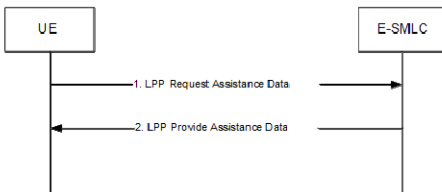
Figure 8.2.3.2.1.2-1: UE-initiated Assistance Data Transfer Procedure
