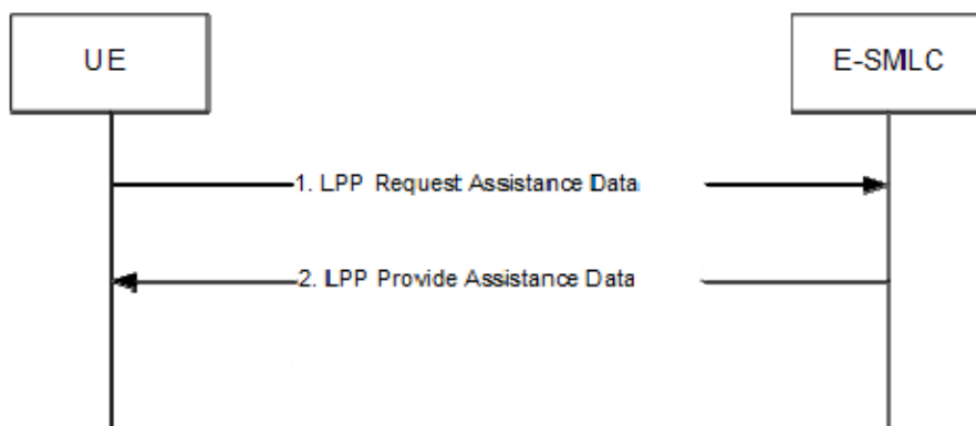
Figure 8.9.3.2.2-1: UE-initiated Assistance Data Transfer Procedure
