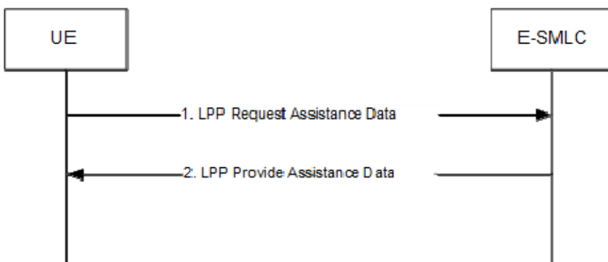
Figure 8.6.3.3.2-1: UE-initiated Assistance Data Transfer Procedure
