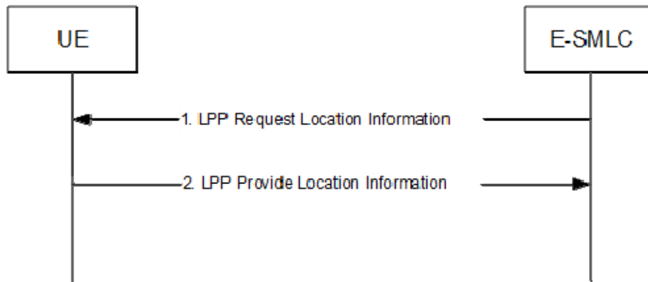
Figure 8.9.3.1.1-1: E-SMLC-initiated Location Information Transfer Procedure
