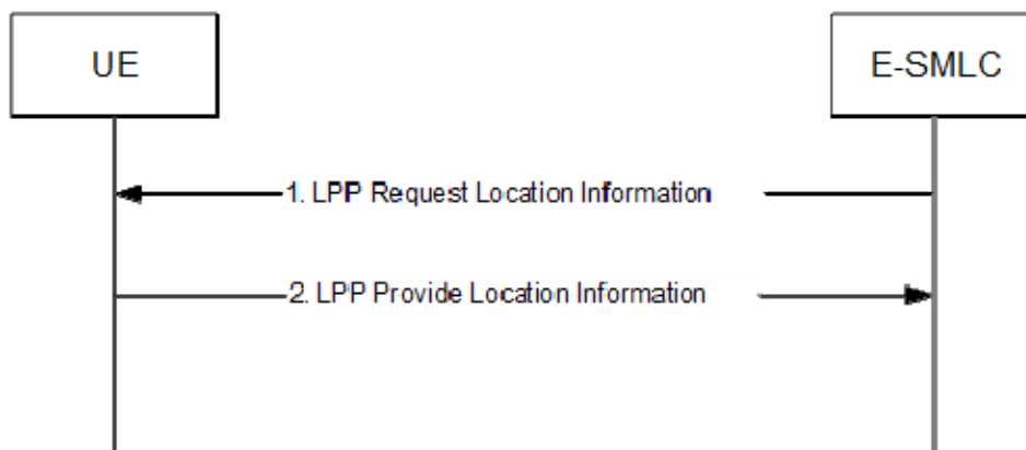
Figure 8.1.3.3.1-1: E-SMLC-initiated Location Information Transfer Procedure
