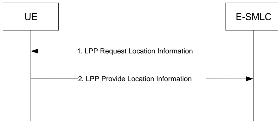
Figure 8.10.3.1-1: E-SMLC-initiated Location Information Transfer Procedure
