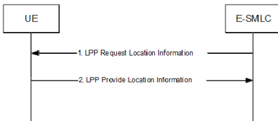
Figure 8.3.3.3.1-1: E-SMLC-initiated Location Information Transfer Procedure.
