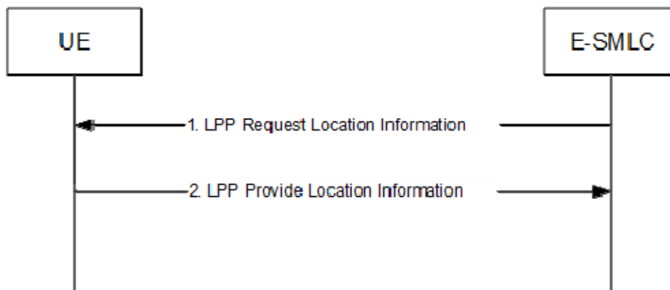
Figure 8.7.3.1.1-1: E-SMLC-initiated Location Information Transfer Procedure
