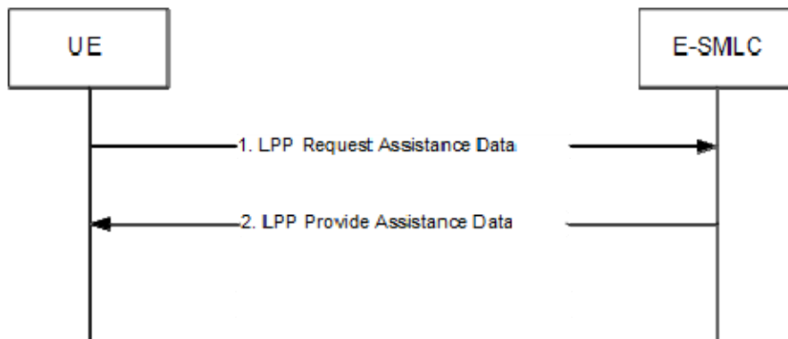
Figure 8.2.3.2.1.2-1: UE-initiated Assistance Data Transfer Procedure
