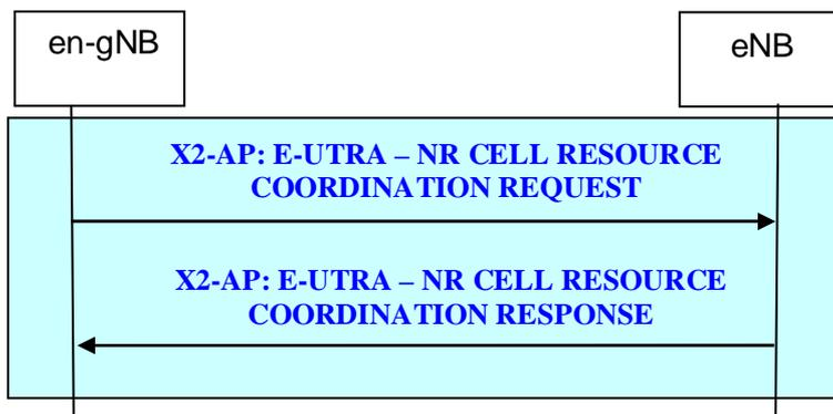
Figure 20.2.2.31-2: E-UTRA - NR Cell Resource Coordination procedure triggered by the en-gNB.
