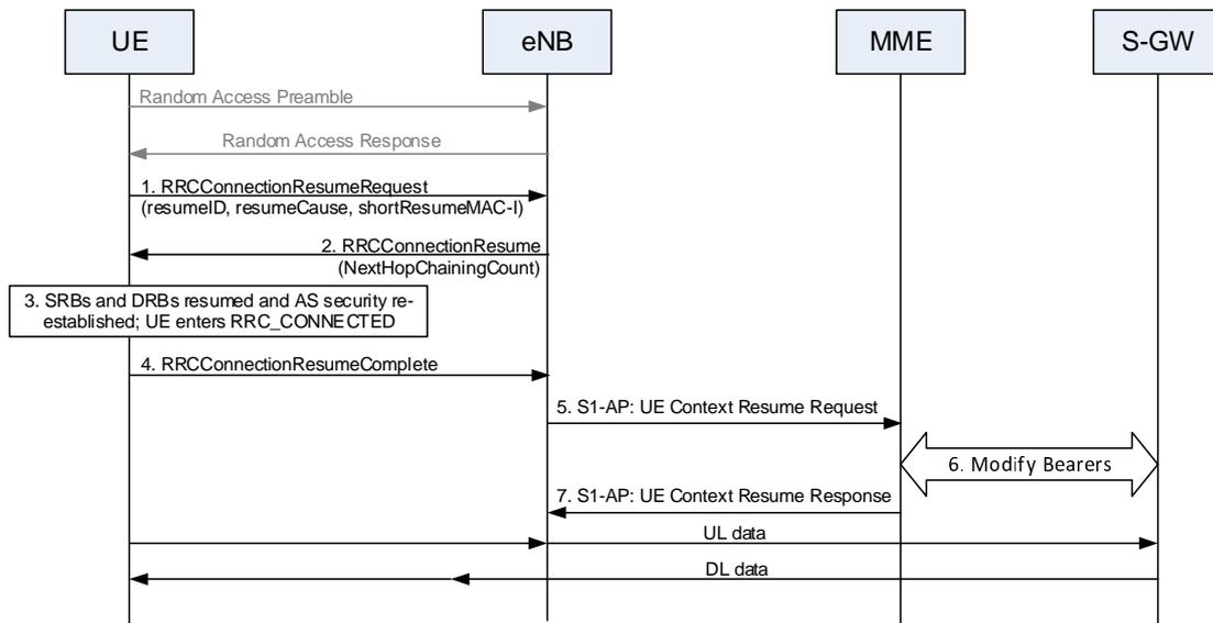
Figure 7.3a.3-2: RRC Connection Resume procedure in EPS
