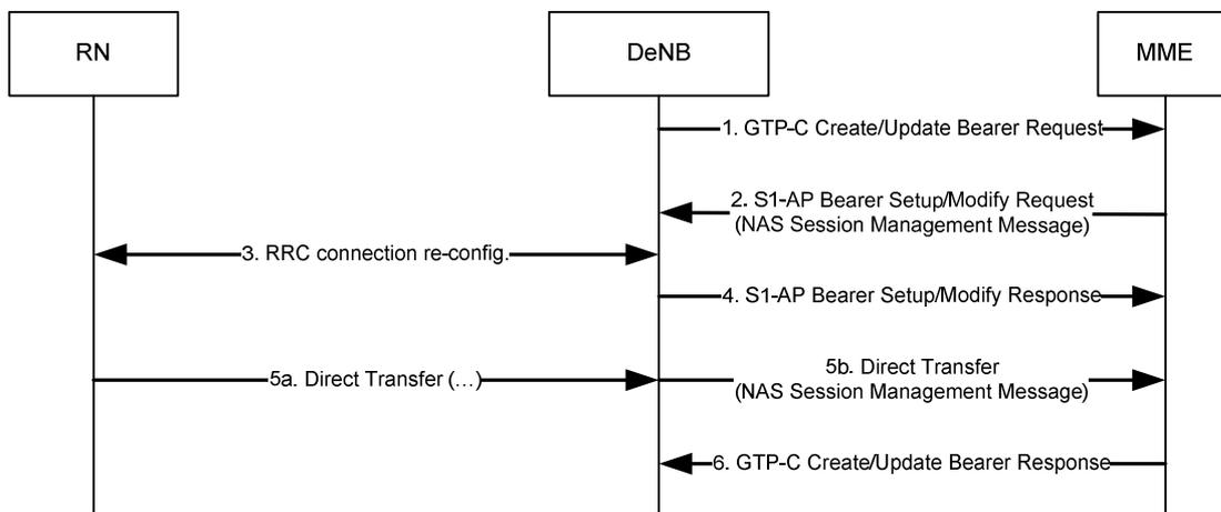
Figure 4.7.6.2-1: DeNB-initiated bearer activation/modification procedure
