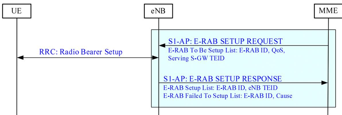
Figure 19.2.2.4.1-1: E-RAB Setup procedure
