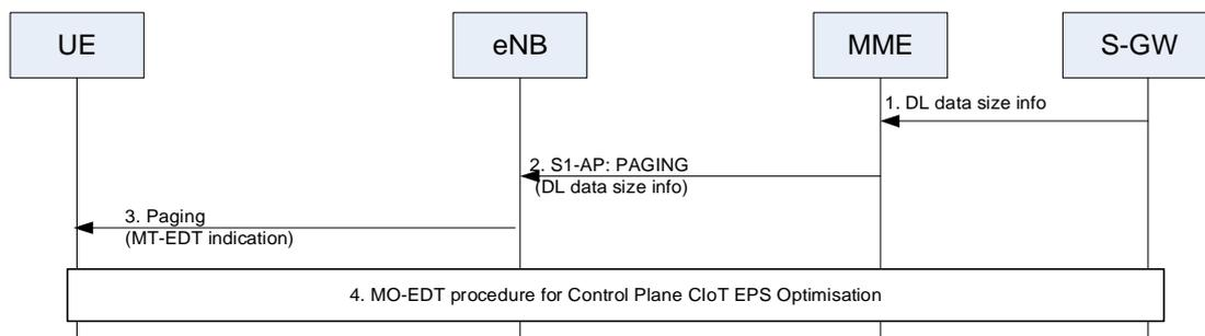
**Figure 7.3c-1: MT-EDT for Control Plane CIoT EPS Optimisation**
