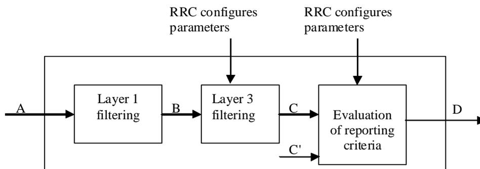
**Figure 10.6-1: Measurement model**
