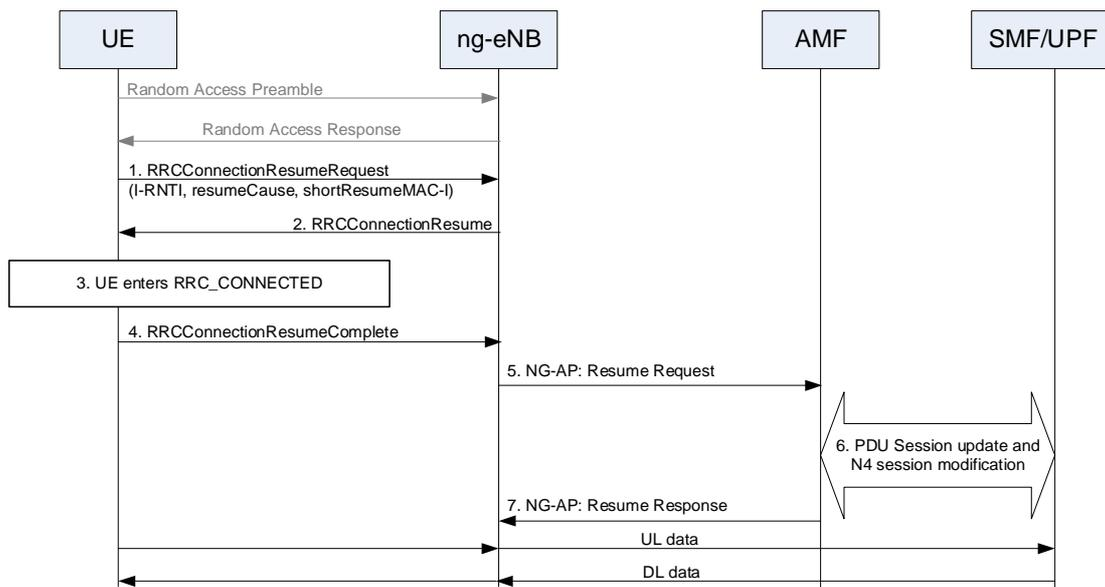
Figure 7.3a.3-2a: RRC Connection Resume procedure in 5GS
