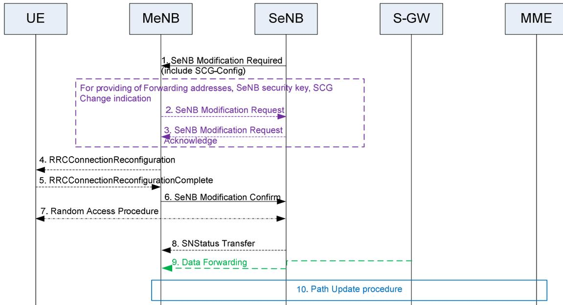
**Figure 10.1.2.8.2-2: SeNB Modification procedure - SeNB initiated**
