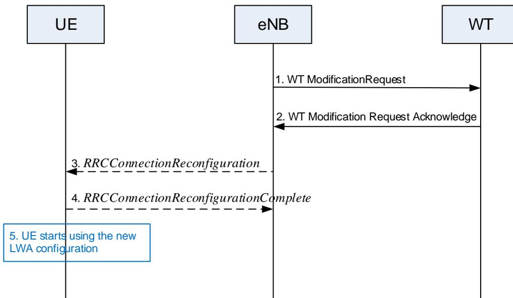
**Figure 22A.1.7.2-1: WT Modification procedure – eNB initiated**
