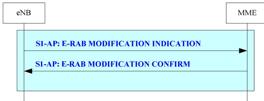
**Figure 19.2.2.4.5-1: E-RAB Modification Indication procedure**
