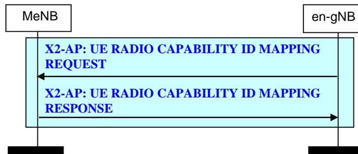
Figure 20.2.2.33-1: UE Radio Capability ID Mapping procedure
