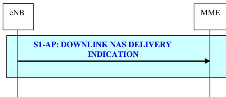
**Figure 19.2.2.6-5: Downlink NAS Delivery Indication procedure**
