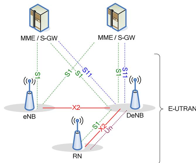
**Figure 4.7.2-1: Overall E-UTRAN Architecture supporting RNs**
