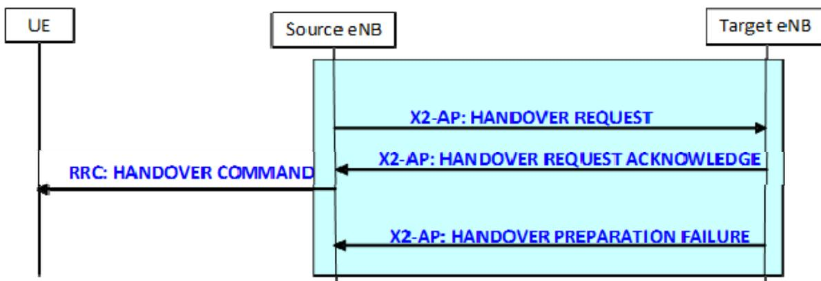
**Figure 20.2.2.1-1: Handover Preparation procedure**
