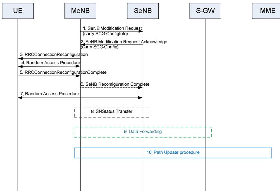
Figure 10.1.2.8.2.1-1: Intra-MeNB handover procedure with SeNB configuration
