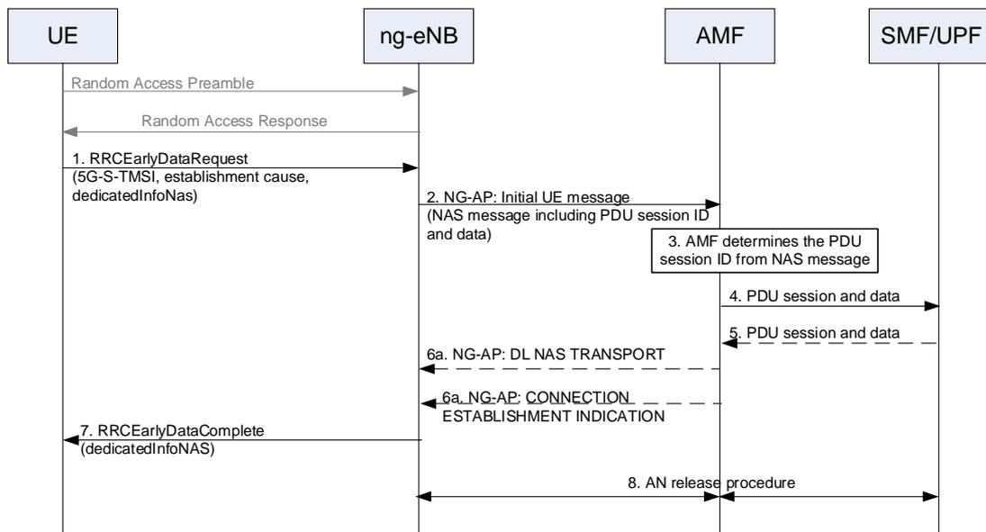
**Figure 7.3b-1a: MO-EDT for Control Plane Clot 5GS Optimisation**
