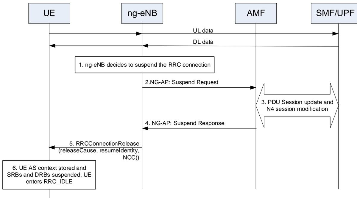
Figure 7.3a.3-1a: RRC Connection Suspend procedure in 5GS
