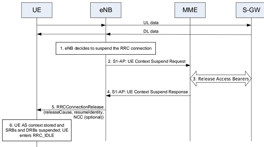
Figure 7.3a.3-1: RRC Connection Suspend procedure in EPS
