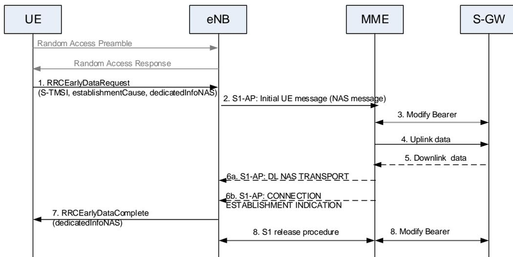
Figure 7.3b-1: MO-EDT for Control Plane ClIoT EPS Optimisation
