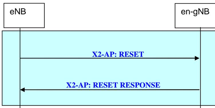
Figure 20.2.2.9-2: eNB-initiated Reset procedure between eNB and en-gNB
