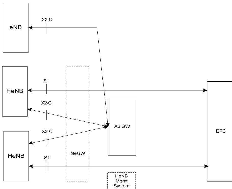
**Figure 4.6.6-1: E-UTRAN operating with X2 GW - Logical Architecture**
