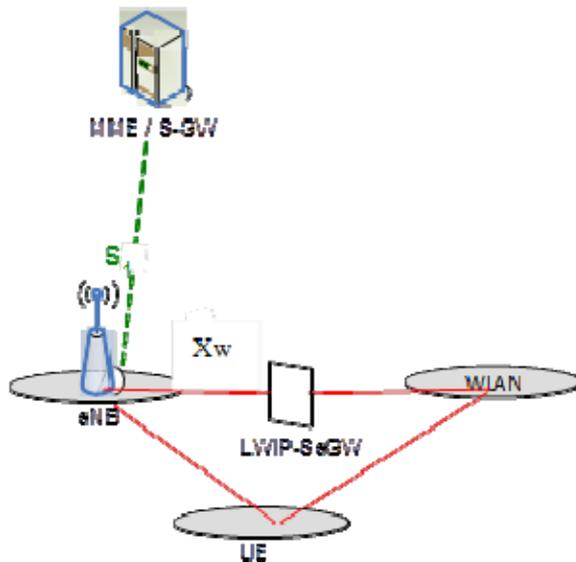
Figure 22A.3-1: LWIP Overall Architecture
