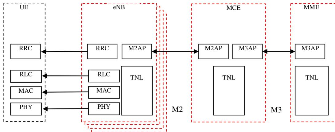
**Figure 15.1.3-1: The E-MBMS c-plane architecture**
