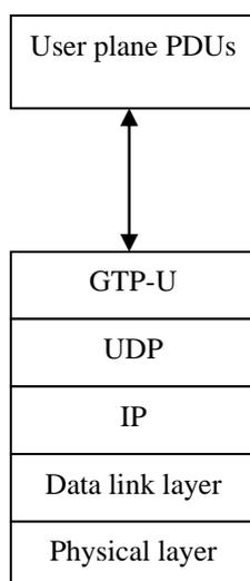
Figure 15.7a.1-1: M1 Interface User Plane (eNB – MBMS GW)
