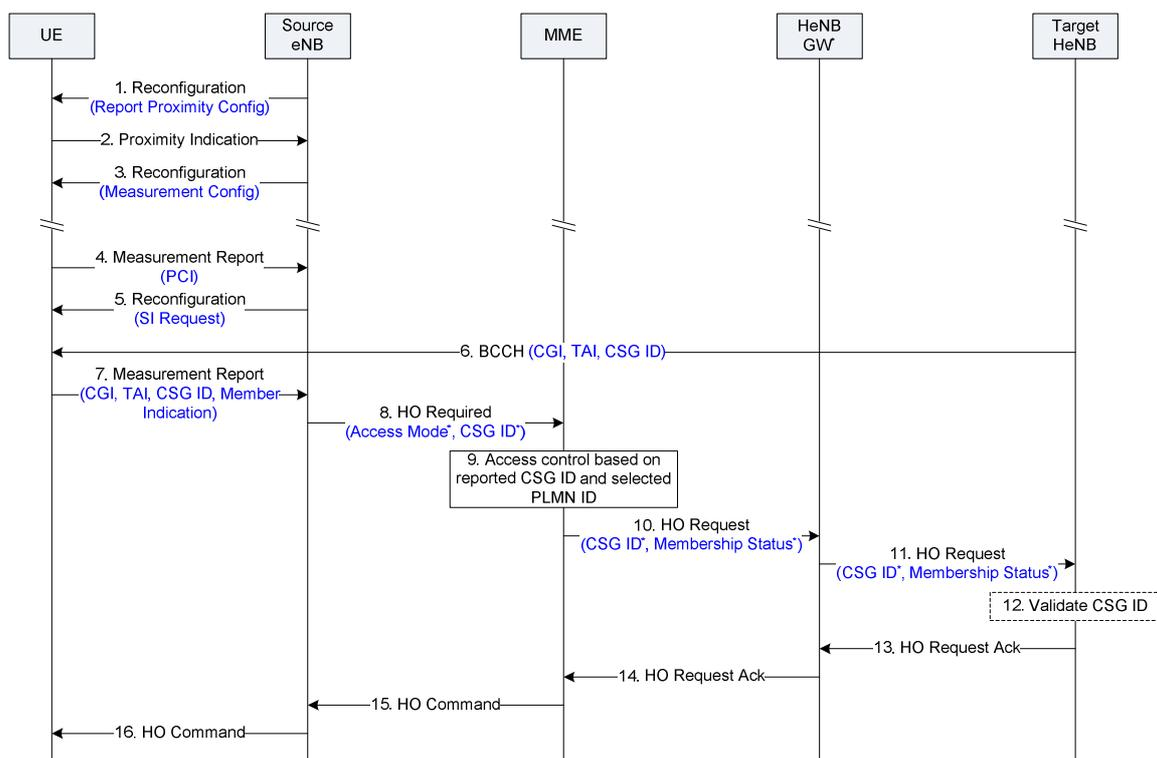
Figure 10.5.1.2-1: Mobility to HeNB's CSG and hybrid cells.
