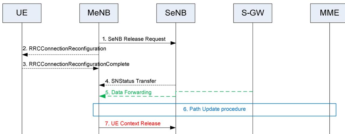
**Figure 10.1.2.8.3-1: SeNB Release procedure – MeNB initiated**
