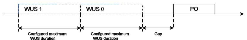
Figure 10.1.4-2: Illustration of GWUS timing for NB-IoT UEs
