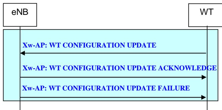
**Figure 22B.2.2.10-1: WT Configuration Update procedure**
