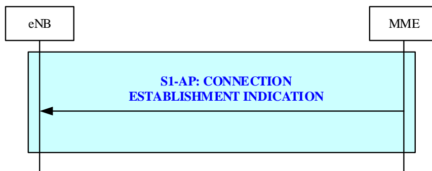
Figure 19.2.25-1: Connection Establishment Indication procedure
