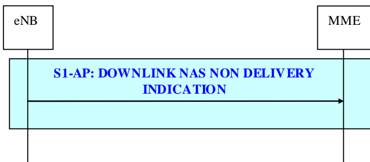
Figure 19.2.2.6-4: Downlink NAS Non Delivery Indication procedure
