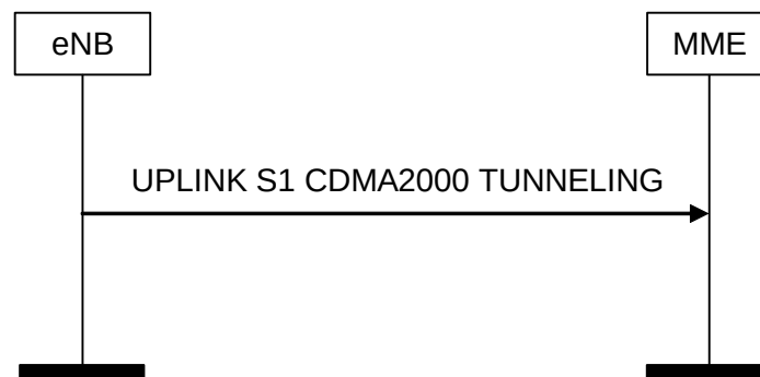
Figure 19.2.2.16.2-1: Uplink S1 CDMA2000 Tunnelling procedure
