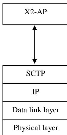
Figure 20.2-1: X2 Interface Control Plane
