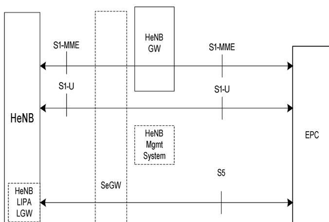
**Figure 4.6.5-1: E-UTRAN - HeNB operating in LIPA mode - Logical Architecture**
