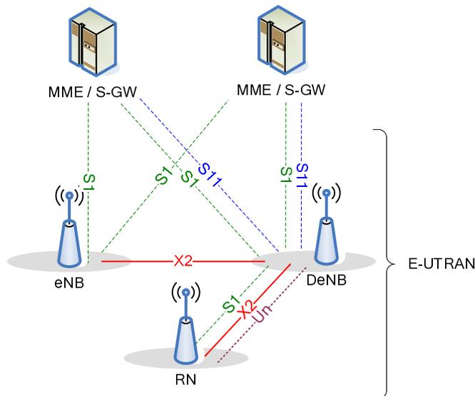
Figure 4.7.2-1: Overall E-UTRAN Architecture supporting RNs
