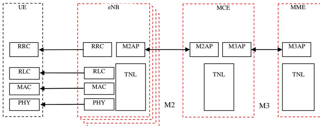
**Figure 15.1.3-1: The E-MBMS c-plane architecture**
