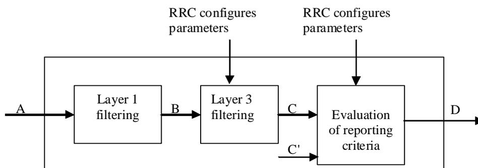
Figure 10.6-1: Measurement model
