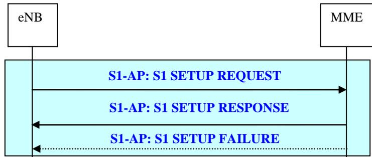
**Figure 19.2.2.8-1: S1 Setup procedure**
