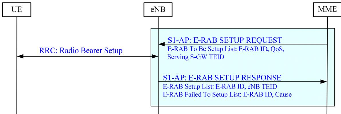
Figure 19.2.2.4.1-1: E-RAB Setup procedure
