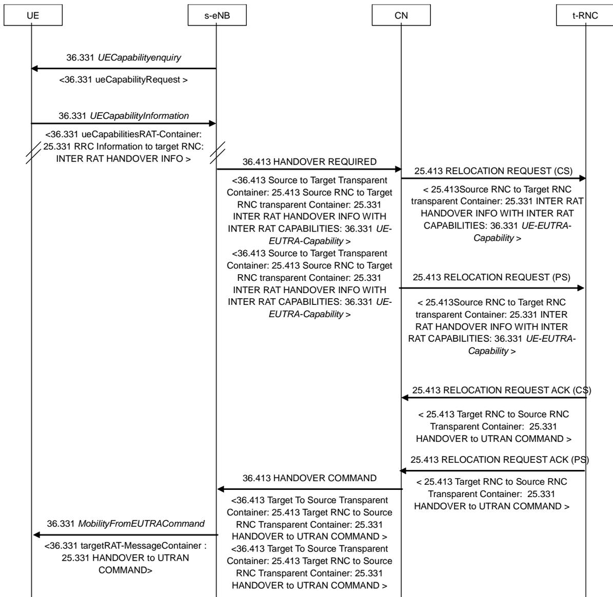
Figure 19.2.2.5.6-7. Handover of PS and CS domain service from EUTRAN to UTRAN, normal flow
