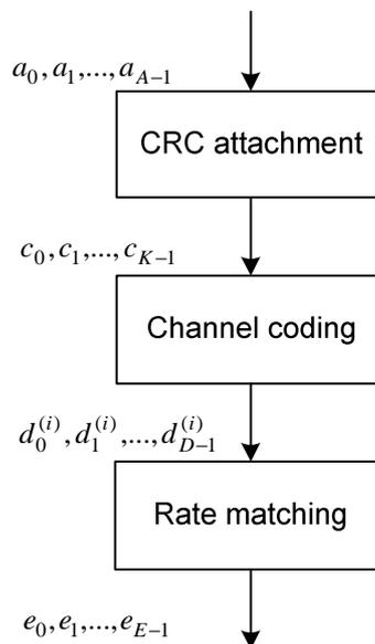
**Figure 6.3.2-1: Transport block processing for UL-SCH**
