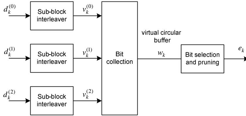
**Figure 5.1.4-1. Rate matching for turbo coded transport channels**
