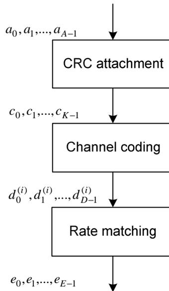
**Figure 5.3.3-1: Processing for one DCI**
