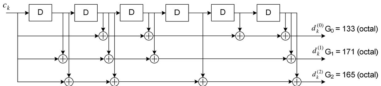
**Figure 5.1.3-1: Rate 1/3 tail biting convolutional encoder**
