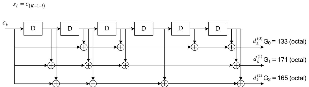
**Figure 5.1.3-1: Rate 1/3 tail biting convolutional encoder.**
