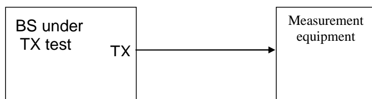
Figure I.1-1: Measuring system Set-up for base station output power, output power dynamics, transmitted signal quality, Frequency error, EVM, DL RS power, Unwanted emissions
