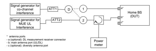
Figure I.1-6: (Option 2) Measuring system set-up for Home BS output power for co-channel E-UTRA protection
