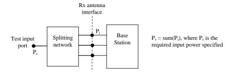
Figure 4.5.7.1-1: Receiver test set-up
