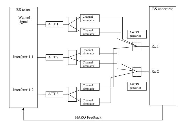
Figure I.3-7b: Functional set-up for enhanced performance requirements type A of PUSCH with 2Rx in multipath fading conditions with asynchronous interference (2 interferers and 2 Rx case shown)
