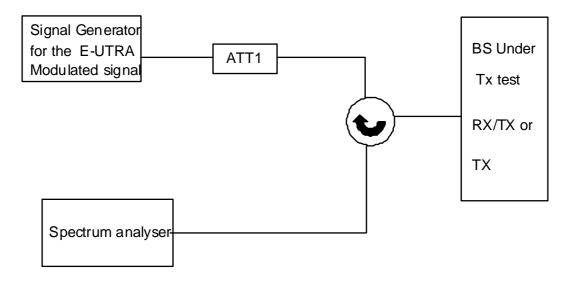
Figure I.1-2: Measuring system Set-up for Transmitter intermodulation
