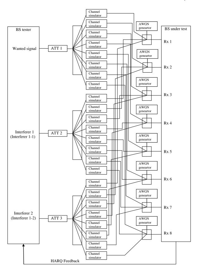
Figure I.3-7d: Functional set-up for enhanced performance requirements type A of 8Rx PUSCH in multipath fading conditions with synchronous or asynchronous interference (2 interferers and 8 Rx case shown)
