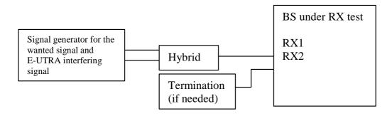
Figure I.2-3: Measuring system Set-up for In-channel selectivity
