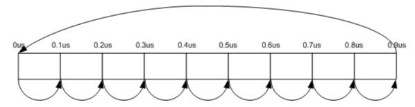
Figure 8.4.1.4.2-2: Timing offset scheme
