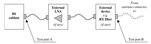
Figure 4.5-2: Receiver test ports
