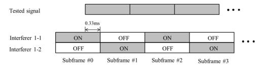
Figure B.6.3-1: Configuration of asynchronous interferers
