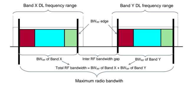
Figure 3.2-1: Illustration of Maximum Radio Bandwidth BW<sub>max</sub> and Total RF Bandwidth BW<sub>tot</sub> for multi-band base station
