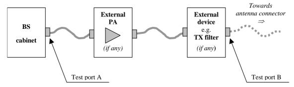
Figure 4.5-1: Transmitter test ports
