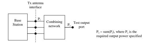
Figure 4.5.7.2-1: Transmitter test set-up
