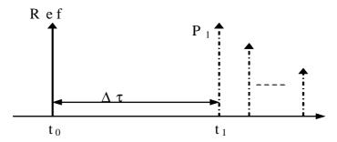
Figure B.4-1: Moving propagation conditions
