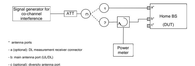
Figure I.1-5: (Option 1) Measuring system set-up for Home BS output power for co-channel E-UTRA protection
