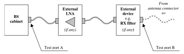
Figure 4.5-2: Receiver test ports
