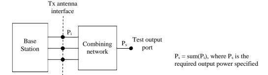
Figure 4.5.7.2-1: Transmitter test set-up
