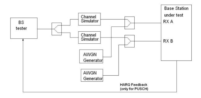
Figure I.3-2: Functional set-up for performance requirements for PUSCH, PRACH, single user PUCCH in multipath fading conditions and for High Speed Train conditions for BS with Rx diversity (2 Rx case shown)
