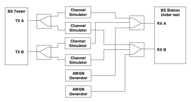
Figure I.3-5: Functional set-up for performance requirements for PUCCH transmission on two antenna ports in multipath fading conditions (2 Rx case shown)
