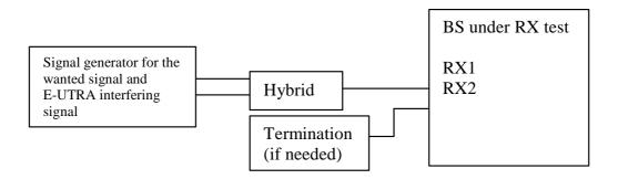
Figure I.2-3: Measuring system Set-up for In-channel selectivit
