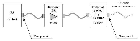
Figure 4.5-1: Transmitter test ports
