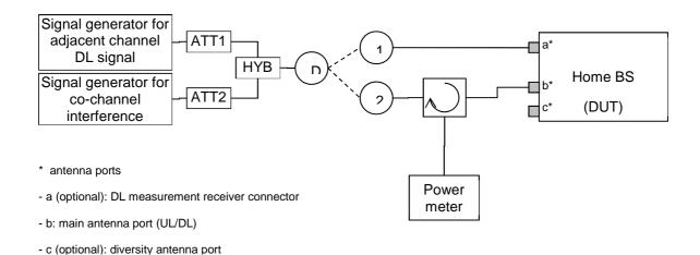
Figure I.1-4: Measuring system set-up for Home BS output power for adjacent channel protection
