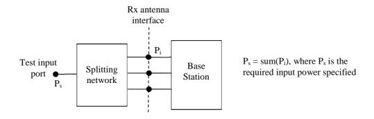
Figure 4.5.7.1-1: Receiver test set-up
