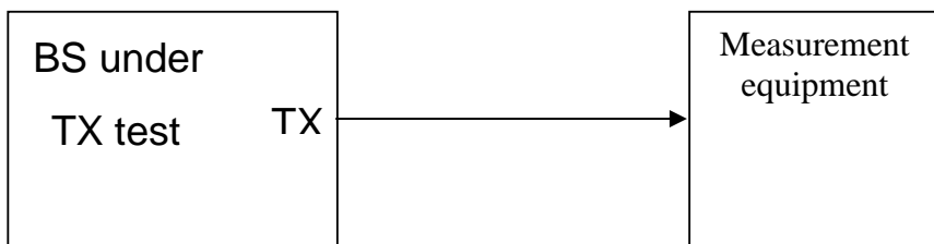
Figure I.1-1: Measuring system Set-up for base station output power, output power dynamics, transmitted signal quality, Frequency error, EVM, DL RS power, Unwanted emissions
