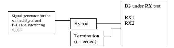
Figure I.2-3: Measuring system Set-up for In-channel selectivity
