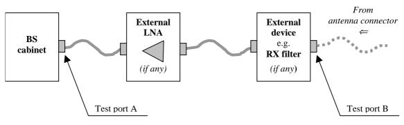
Figure 4.5-2: Receiver test ports
