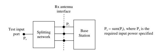
Figure 4.5.7.1-1: Receiver test set-up
