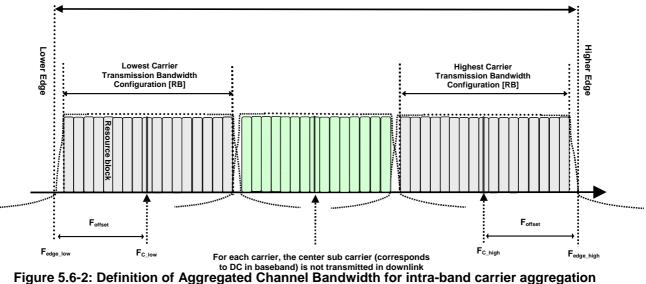
The lower edge of the Aggregated Channel Bandwidth ( $BW_{Channel\_CA}$ ) is defined as  $F_{edge\_low} = F_{C\_low} - F_{offset}$ . The upper edge of the aggregated channel bandwidth is defined as  $F_{edge\_high} = F_{C\_high} + F_{offset}$ . The Aggregated Channel Bandwidth,  $BW_{Channel\_CA}$ , is defined as follows:
