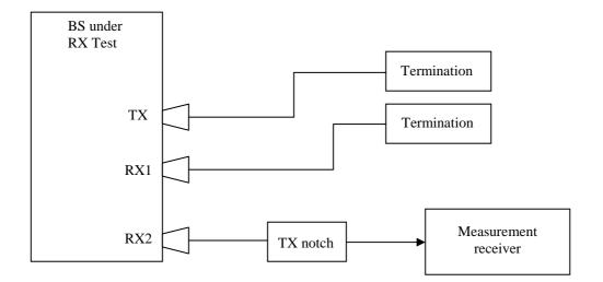
Figure I.2-6: Measuring system Set-up for Receiver spurious emission
