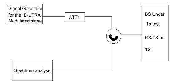
Figure I.1-2: Measuring system Set-up for Transmitter intermodulation
