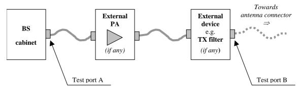
Figure 4.5-1: Transmitter test ports
