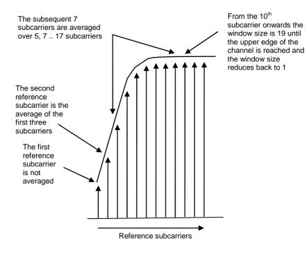
Figure F.3.4-1: Reference subcarrier smoothing in the frequency domain
