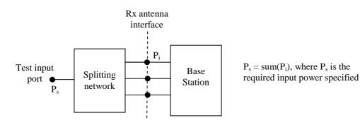
Figure 4.5.7.1-1: Receiver test set-up
