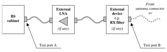
Figure 4.5-2: Receiver test ports
