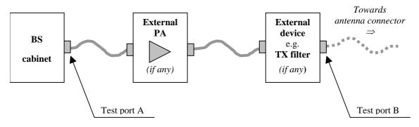
Figure 4.5-1: Transmitter test ports
